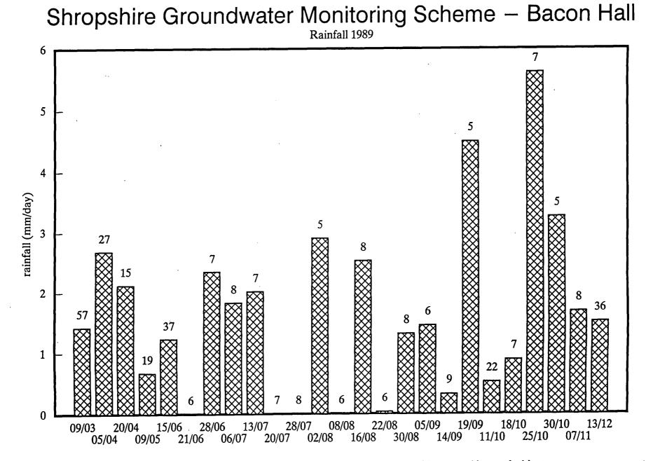
Figure 2 Rainfall 1989, Bacon Hall site. Rainfall expressed as mm/day over the period between measurements - no. of days between measurements is given at the top of the each bar.
