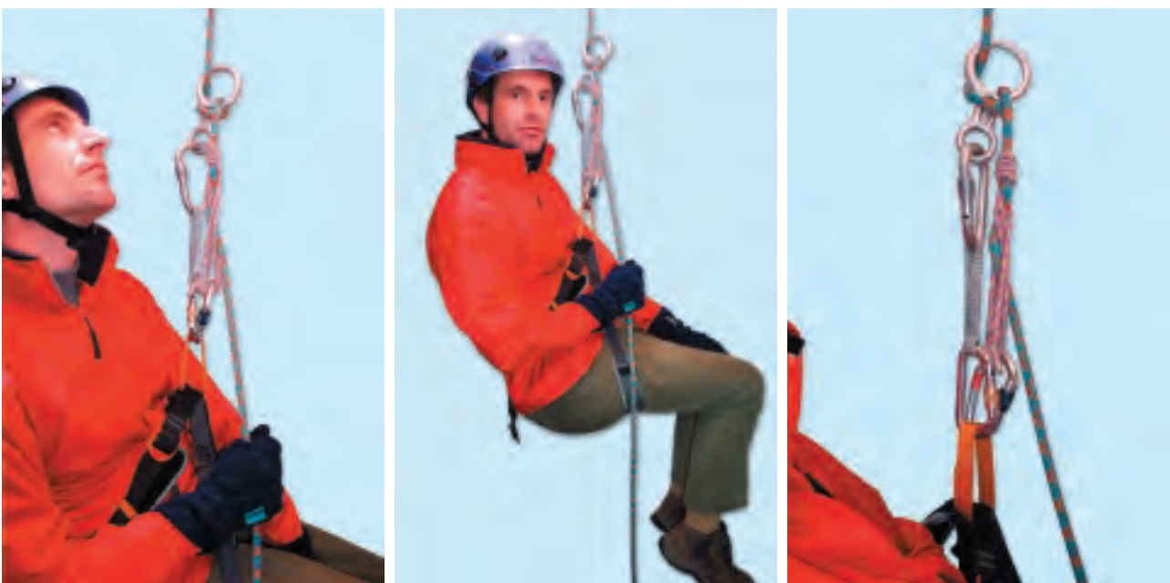
Figure 10.11 The BAS abseil system
