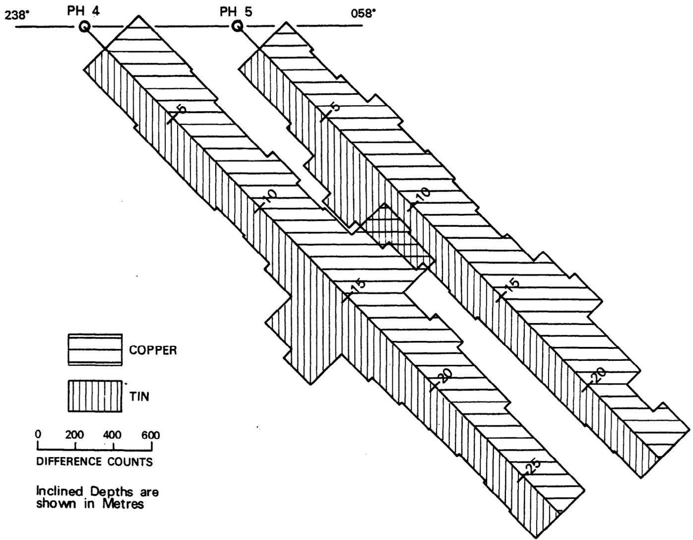
Fig. 12 Portable XRF Measurements on Pulps from PH 4 and PH 5
