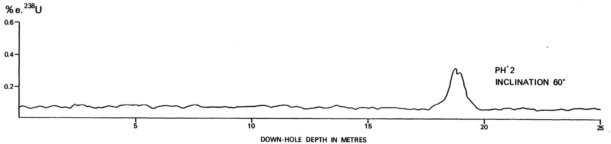
Fig. 9 Geiger-Müller logs of percussion holes : PH 1 and PH 2
