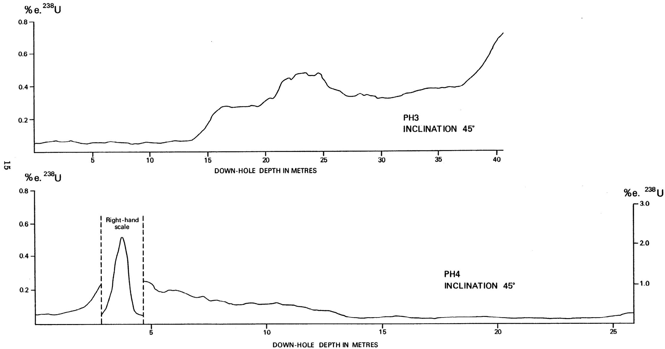
Fig. 10 Geiger - Müller logs of percussion holes : PH 3 and PH 4
