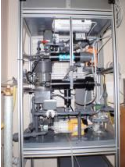
Ferrybox system for continuous measurements as installed on the RV Cefas Endeavour
