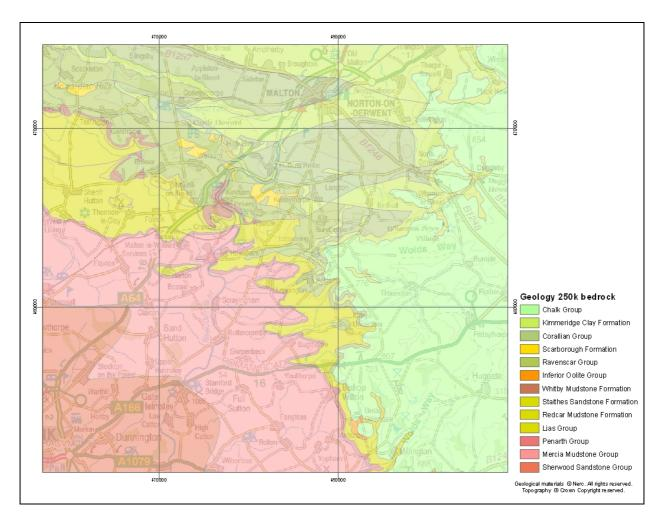
Figure 3. Geology of the Vale of York landslide survey area.
