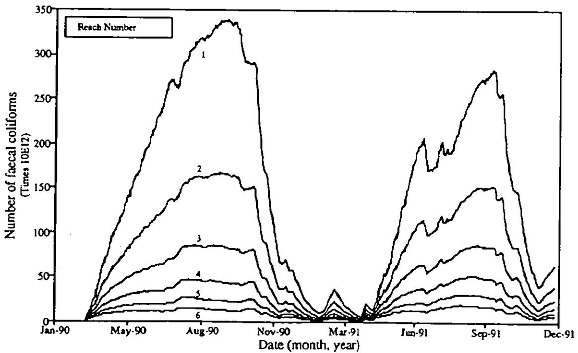
Figure 6.5 Time series of modelled faecal coliform numbers in channel storage for reaches along the River Exe between Thorverton STW and Pynes water intake.
