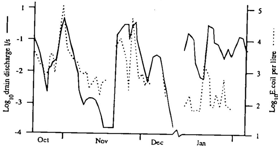
Figure 3.3 Variation of *E. coli* concentration in water draining an extensive land drainage system in the absence of recent inputs of faecal bacteria (after Igneous and Evans, 1972).
