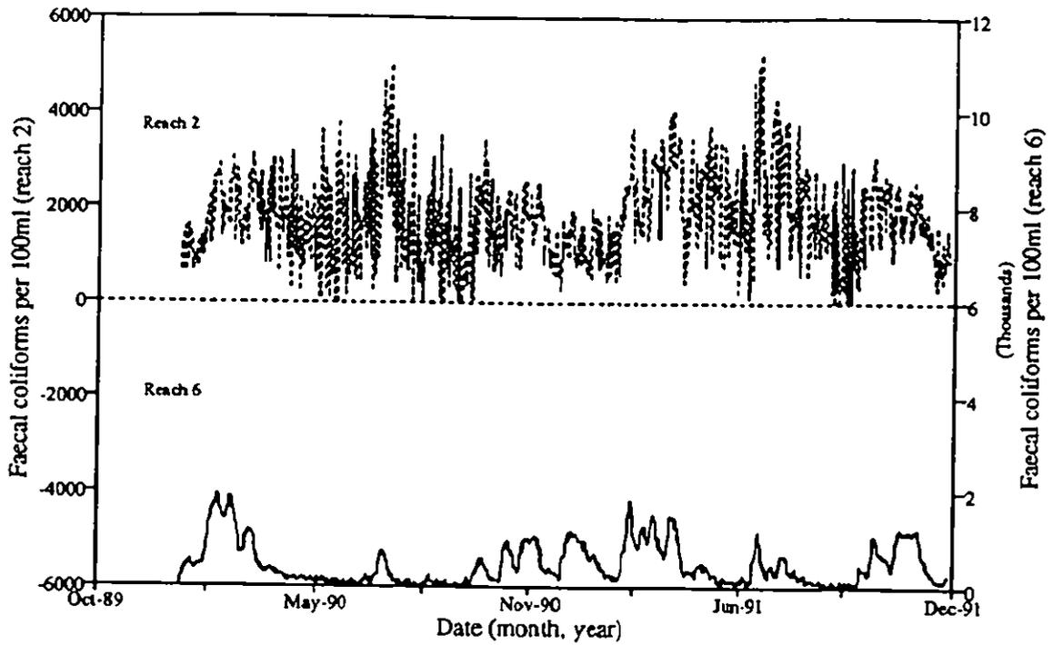
Figure 6.4 Time series of modelled faecal coliform concentration at the output of model reaches 2 and 6; each reach is 1km in length.
