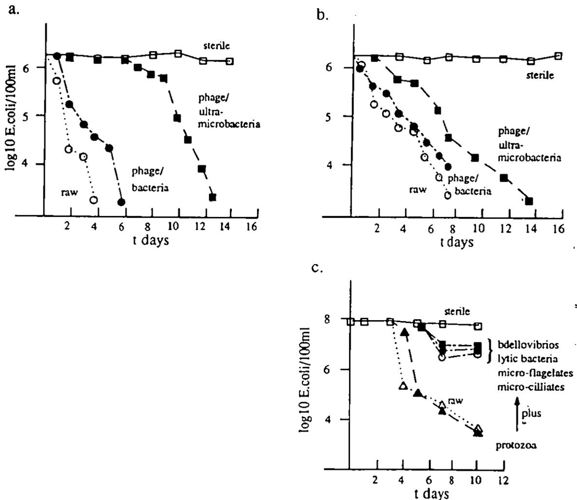
Figure 2.7 The influence of successive removal of sections of natural microbial communities on *E.coli* die-off in a. "clean" river water, b. sewage contaminated river water (after Flint 1987) and c. estuarine water (after Enzinger and Cooper 1976).
