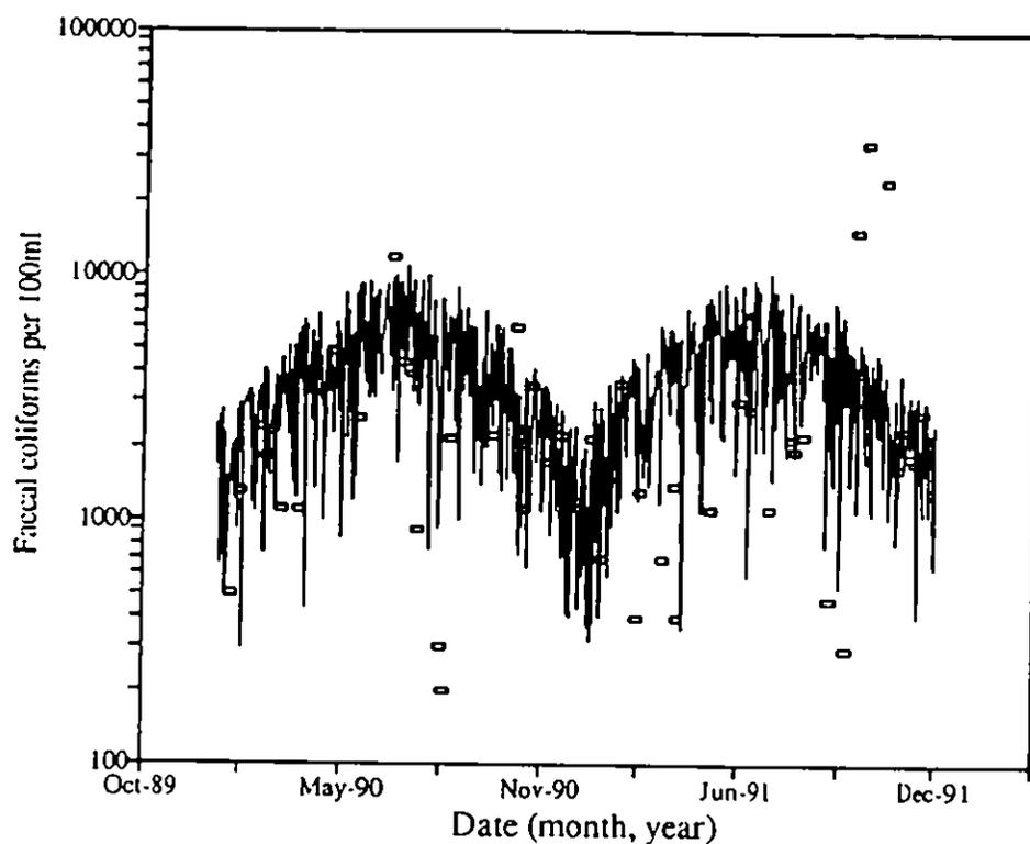
Figure 6.2 Raw data ( $\square$ ) and artificially generated time series (solid line) of faecal coliform concentrations for the River Exe at Thorverton.
