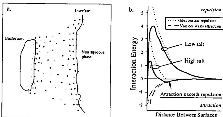
**Figure 3.1** a. Schematic representation of the interaction between potentially overlapping cation clouds accompanying a negatively-charged bacterium as it approaches a negatively-charged interface, b. idealised curves showing the potential energy of interaction as a function of distance between a bacterium and an interface in solutions of different salt concentration (after Marshall 1979).
