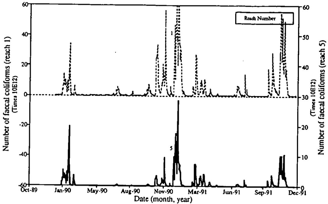
Figure 6.6a Time series of modelled faecal coliform entrainment episodes from channel storage during flow events; reaches 1 and 5 are shown.
