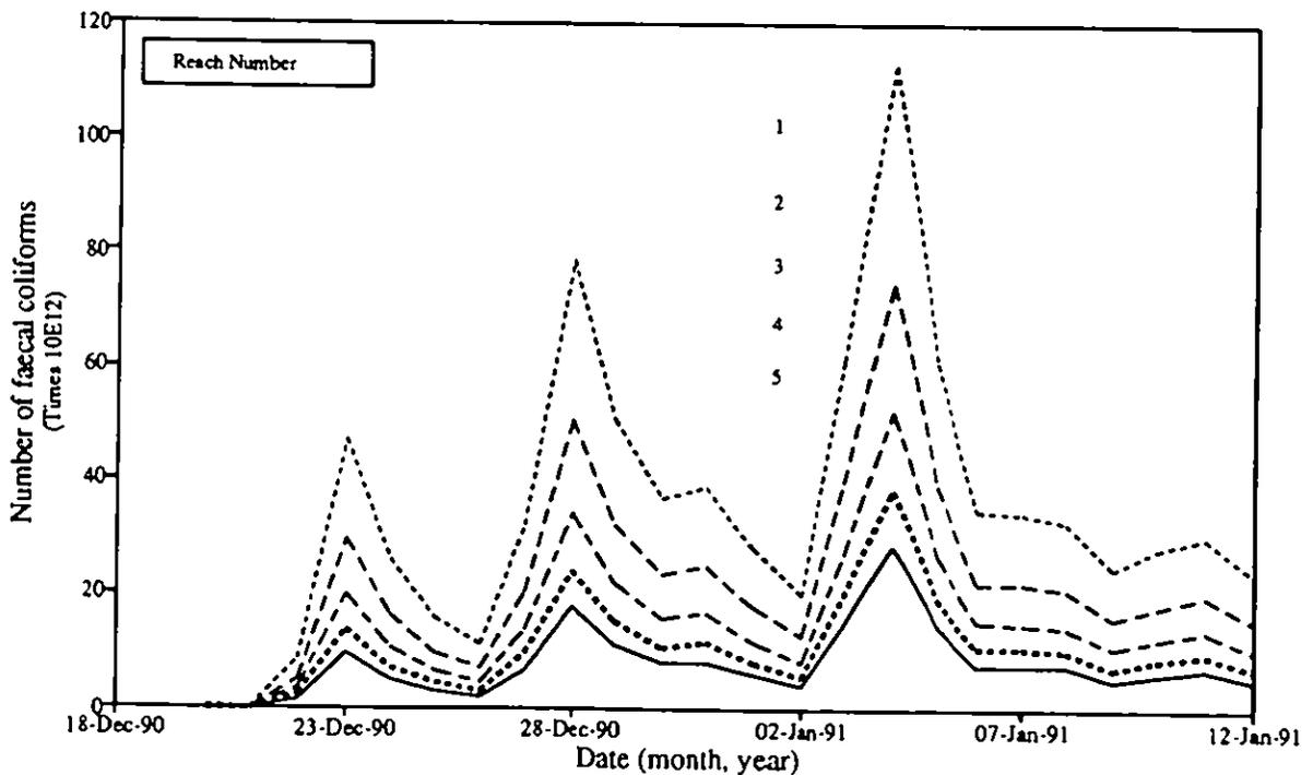
Figure 6.6b Time series of three modelled faecal coliform entrainment episodes over the New Year period 1990-91 in model reaches 1 and 5 of the River Exe between Thorverton STW and Pynes water intake.
