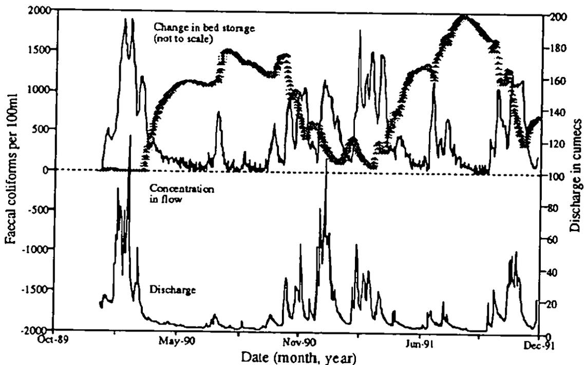
**Figure 6.3a** Time series of flow and modelled faecal coliform concentration and channel storage for the River Exe at Pynes water intake.
