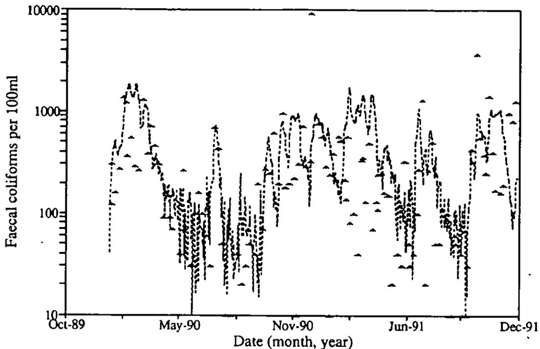
*Figure 6.3b Modelled and observed time series of faecal coliform concentrations for the River Exe at Pynes water intake.*
