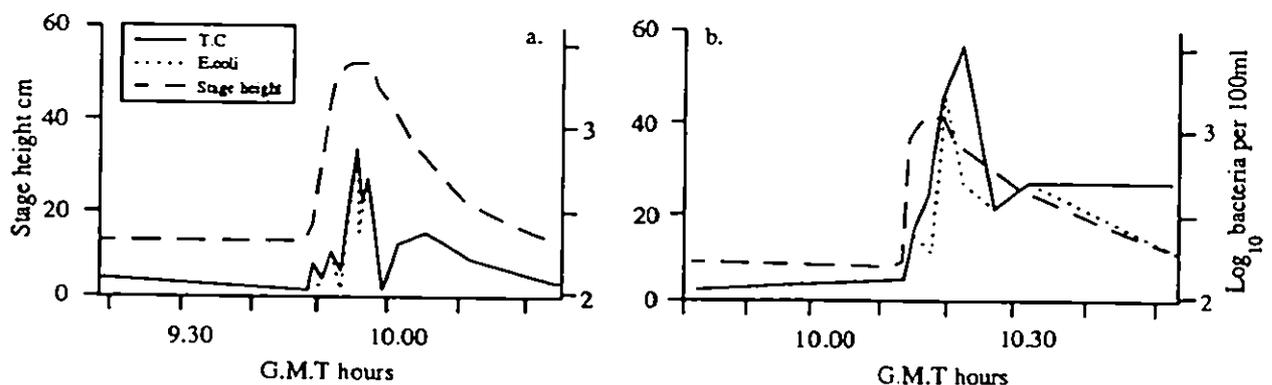
**Figure 3.7** Propagation of artificially generated hydrograph with response of total coliforms (TC) and *E.coli* concentration at locations (a) 400m, and (b) 2500m downstream of the hydrograph source (after McDonald *et al.*, 1982).
