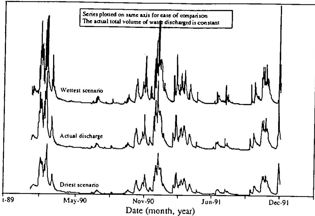
**Figure 6.8** Time series of actual and modified flows in the River Exe at Thorverton. The flows have been modified on the basis of CCIRG projections for the year 2050 (Arnell, 1992).
