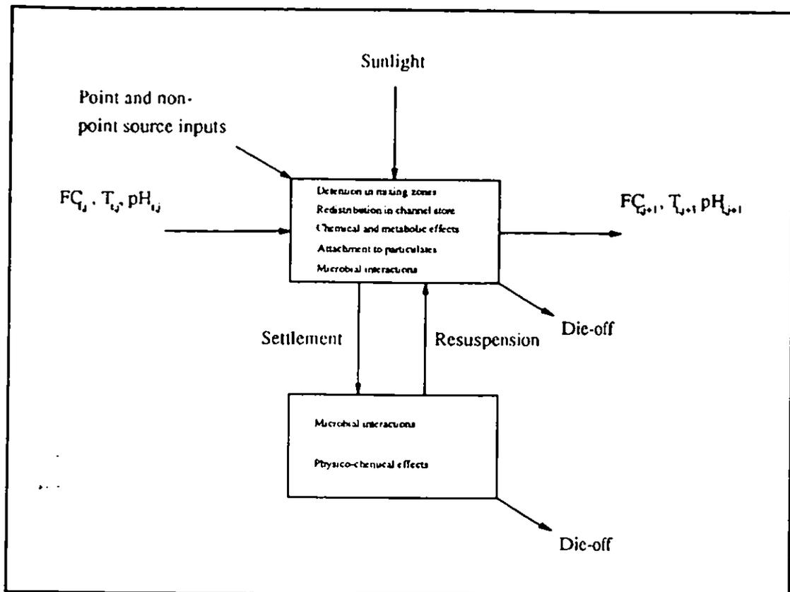
Figure 5.5 Two-box conceptualisation of the faecal coliform model as applied to a single river reach.
