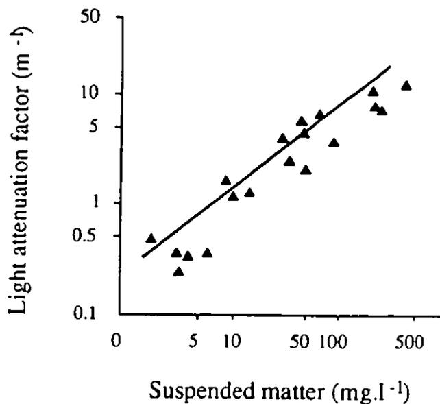
**Figure 2.4** Plot of light attenuation factor,  $\eta$ , per metre depth against suspended matter concentration (after Pommepeuy *et al.* 1992).
