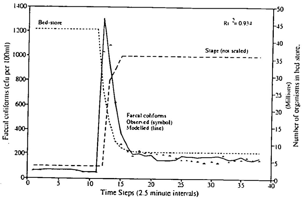
*Figure 5.6a* Observed and modelled faecal coliform concentrations in response to a step change in flow on the River Washburn.  $R_1^2$  is a goodness of fit criterion and should be approaching 1.
