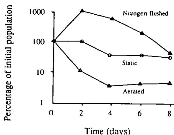
Figure 2.9 Survival of faecal coliform in raw river water at 20°C in aerated, static and N<sub>2</sub> flushed flasks (after Zerfas, 1970).
