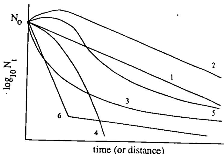
**Figure 4.1** Bacterial die-off curves as predicted by models in the literature (after Crane and Moore, 1986).
