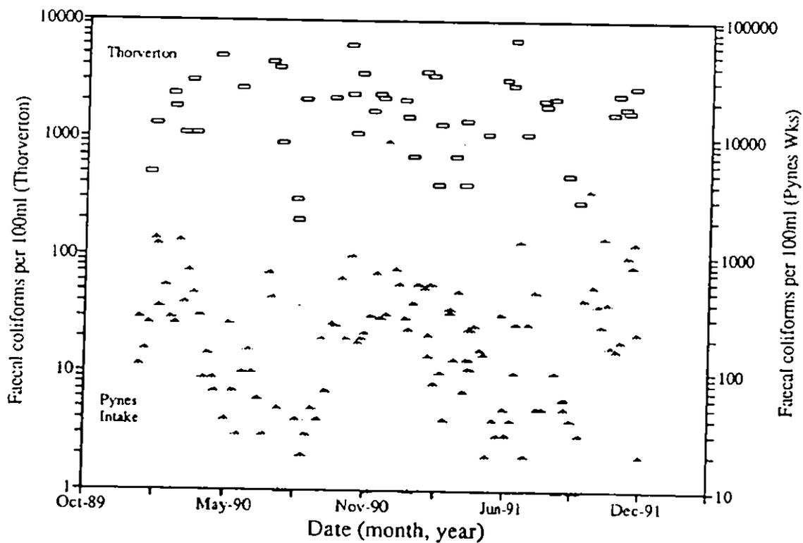
Figure 6.1 Time series of faecal coliform concentrations at Thorverton STW and the Pynes water intake on the River Exe in Devon; data are presented in their raw "as sampled" state.
