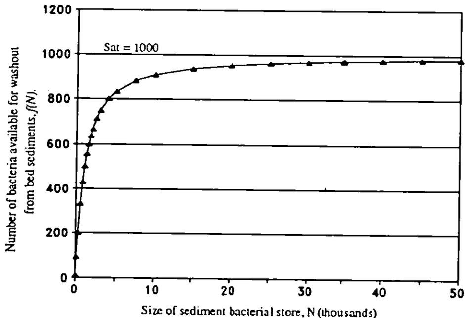
Figure 4.3 Plot of washout limitation function, for  $Sat=1000$ , as given by equation 4.18.
