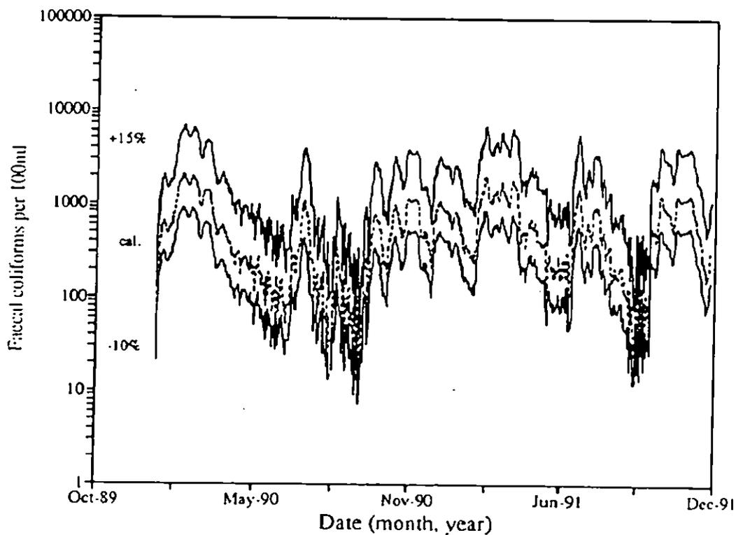
**Figure 6.7** Time series of modelled faecal coliform concentration at Pynes water intake showing the impact of increased and reduced faecal coliform loadings.
