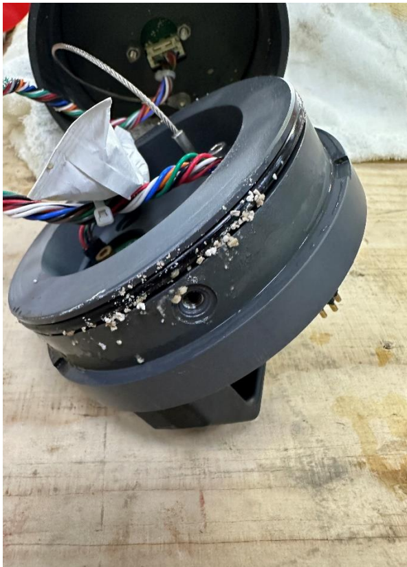
SBE SeaFET with desiccant around o-ring.
