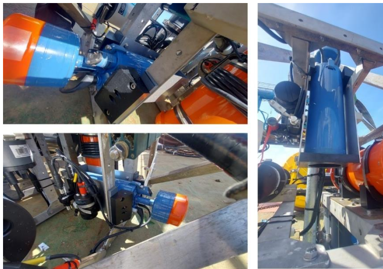
The 30m Seaguard – with bracket, optode and fluorometer
