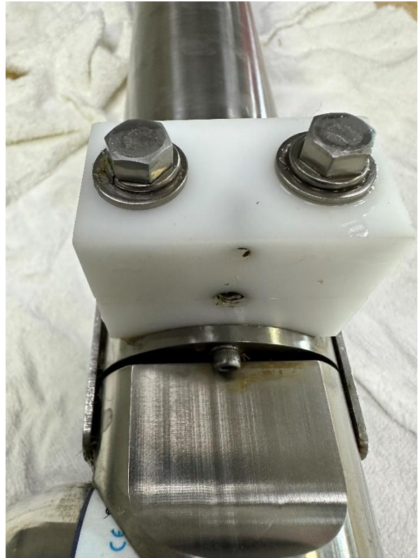
Flooded SBE 37 ODO SN: 23950 Loose pump housing.
