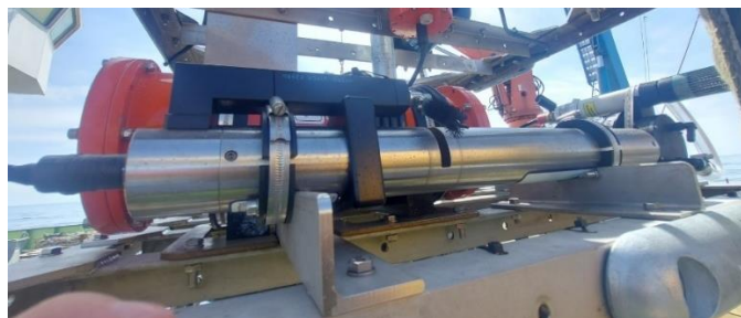
Suna nitrate with brush visible half way along, brush movement checked onboard
