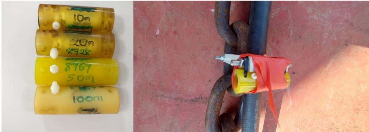
Initial set up and an example of star oddi attached on JC247
