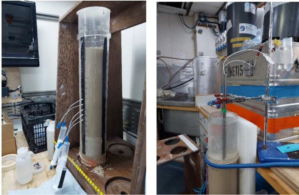
Figure 16.1. Left: Porewater extraction with Rhizones; Right: Lab-on-Chip porewater setup.
