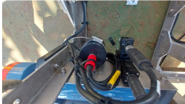
The zebra-tech wiper and motor for the cyclops fluorometer
