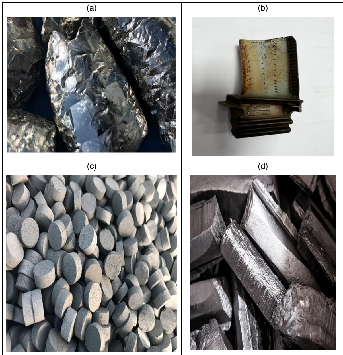
Figure 6. A various forms of material and alloy used in aerospace and defence industries. (a) Hafnium crystal bar, (b) High Pressure Turbine blade with thermal barrier coating, (c) Rhenium pellets and (d) Tantalum ingot. © Advanced Alloy Services Ltd, reproduced with permission
