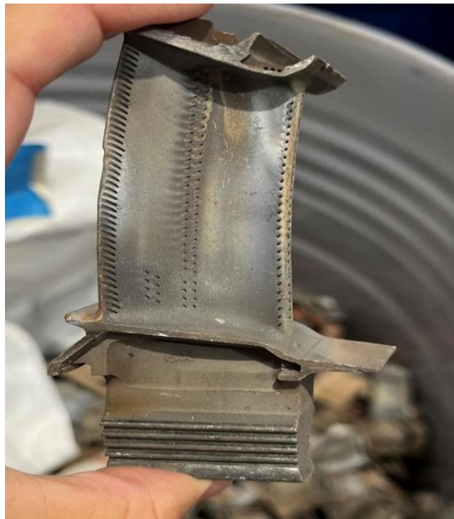
Figure 3. An end-of-life single-crystal turbine blade. The holes in the surface of the blade permit airflow along cooling channels to keep the blade within its specified operating temperature range.
