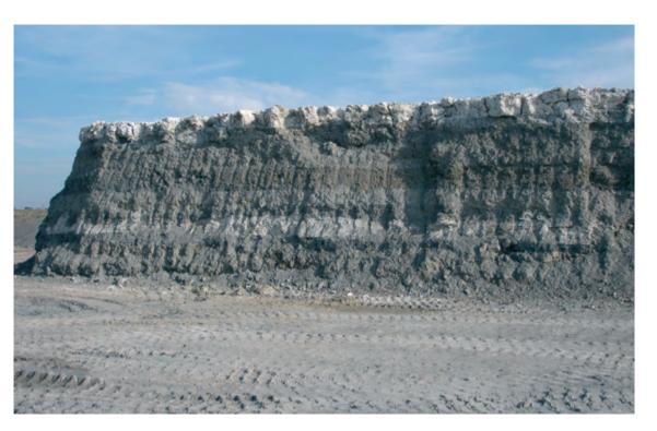
Blending fireclays using layered stockpiles.
