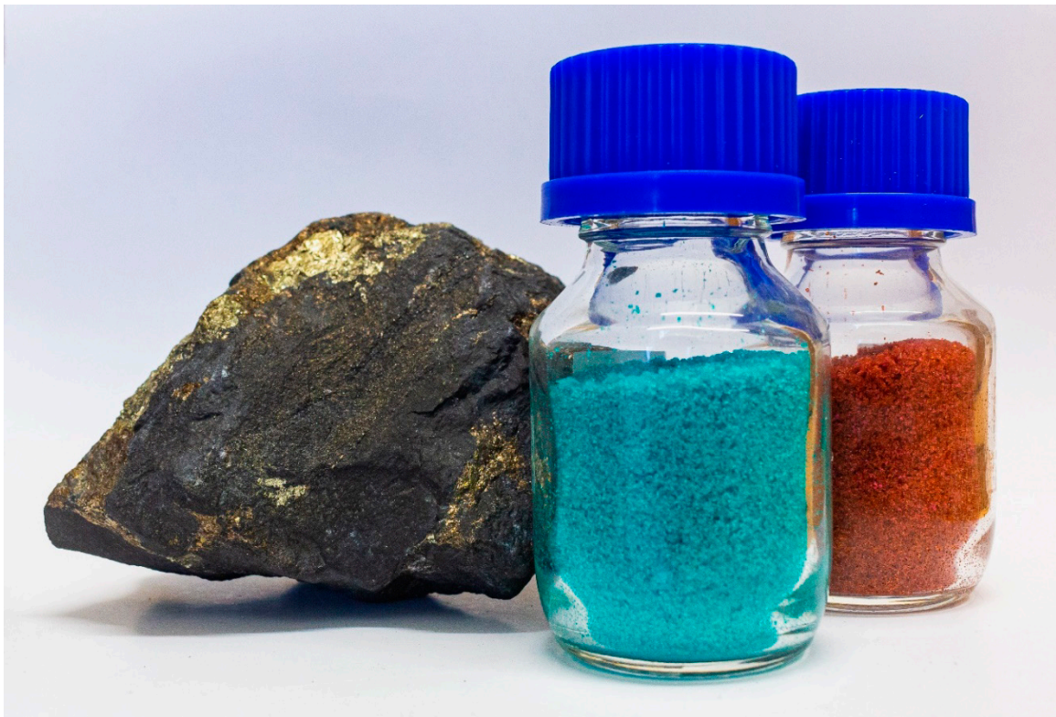
Figure 14 Nickel-copper-cobalt ore and its end-products nickel (blue) and cobalt sulfates (orange) produced at the Sotkamo mine in Finland operated by Terrafame. The mine produces these chemicals used for battery technologies on-site. The Sotkamo mine has the largest cobalt resources and reserves in Europe, that are currently in production (© Terrafame Ltd. 2020 84 ).
