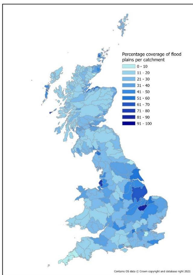
**Figure 8** Catchment Flood Accommodation.
