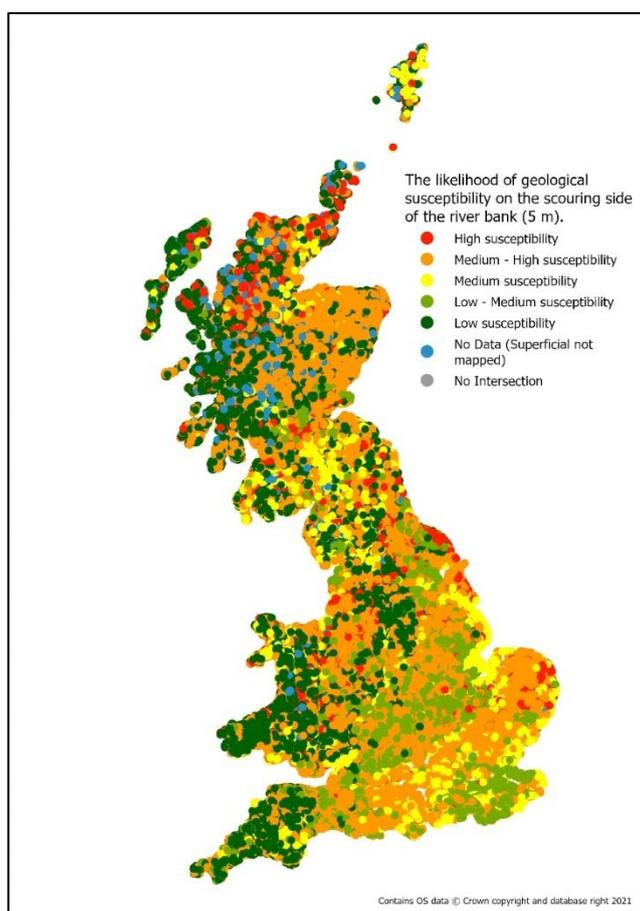
**Figure 17** Lateral River Erosion data.
