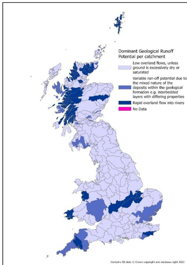
**Figure 13** The dominant geological run-off potential per catchment.
