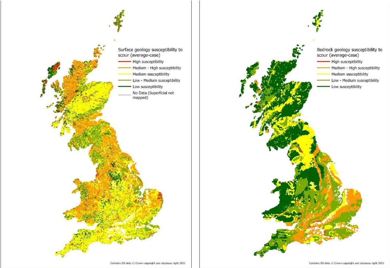
**Figure 16** Surface Geology Susceptibility (left) and Bedrock Geology Susceptibility (right).
