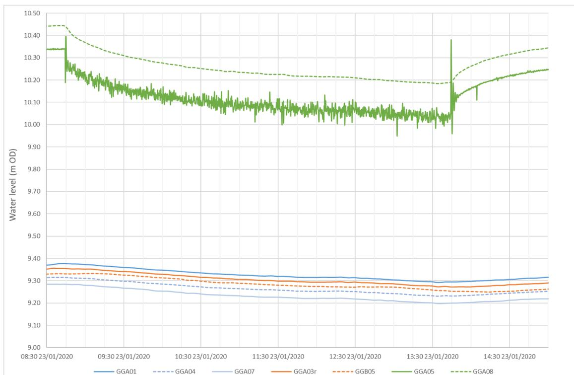
Figure 57 Borehole water levels (from data logger) in pumping and observation boreholes during the CRT on GGA05
