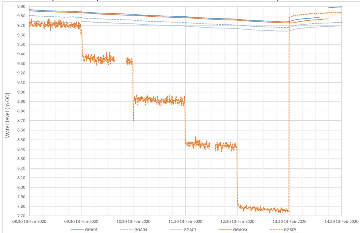
**Figure 32 Borehole water levels (from data logger) in pumping and observation boreholes during the SDT on GGB05**
