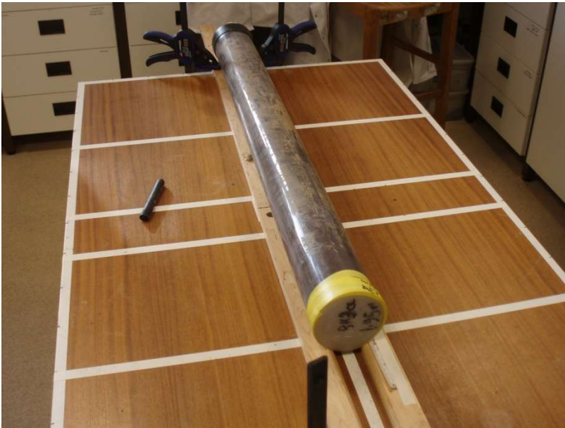
Figure 41 Non-contact resistivity (NCR) table with 1.5 m long core run (BGS, Keyworth)
