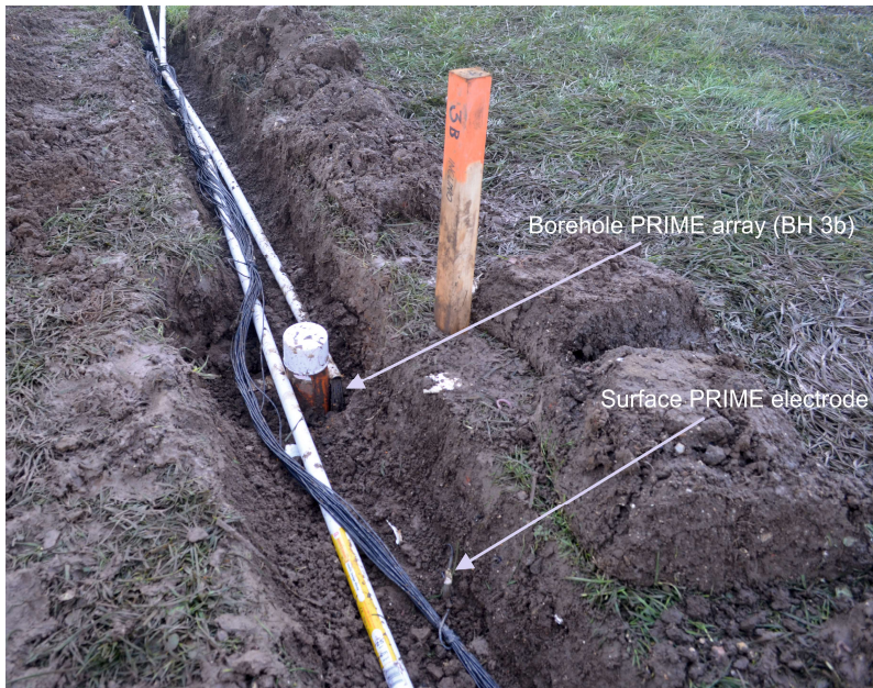
Figure 36 Trench containing PRIME surface resistivity array and borehole resistivity array trailing cables emerging from Borehole 3b.
