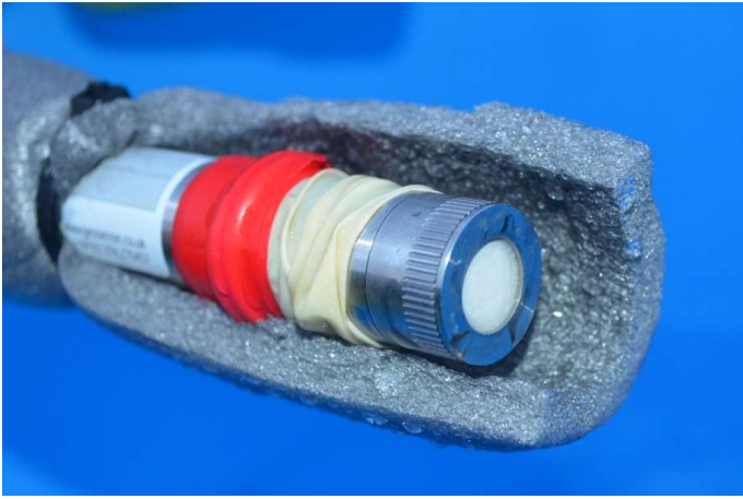
Figure 31 Piezometer sensor showing push-on cap containing high air-entry sintered alumina filter
