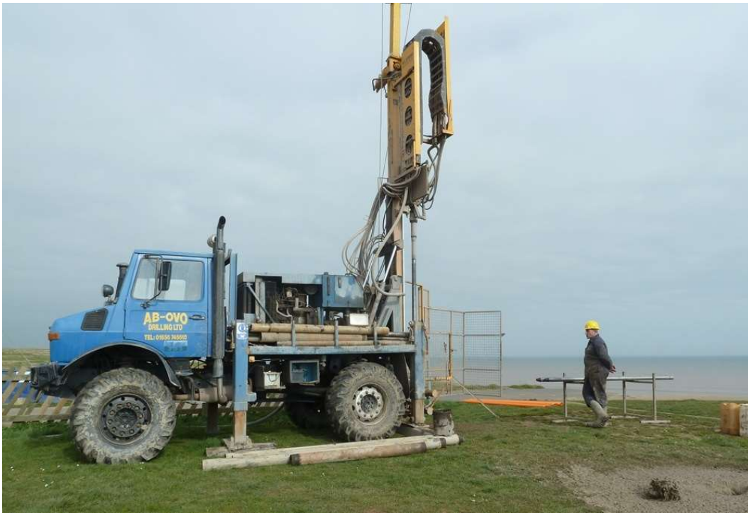
Figure 7 Unimog-Klemm rotary drilling rig at borehole 1b (Photo: C. Spalton, MGS-Geosense)
