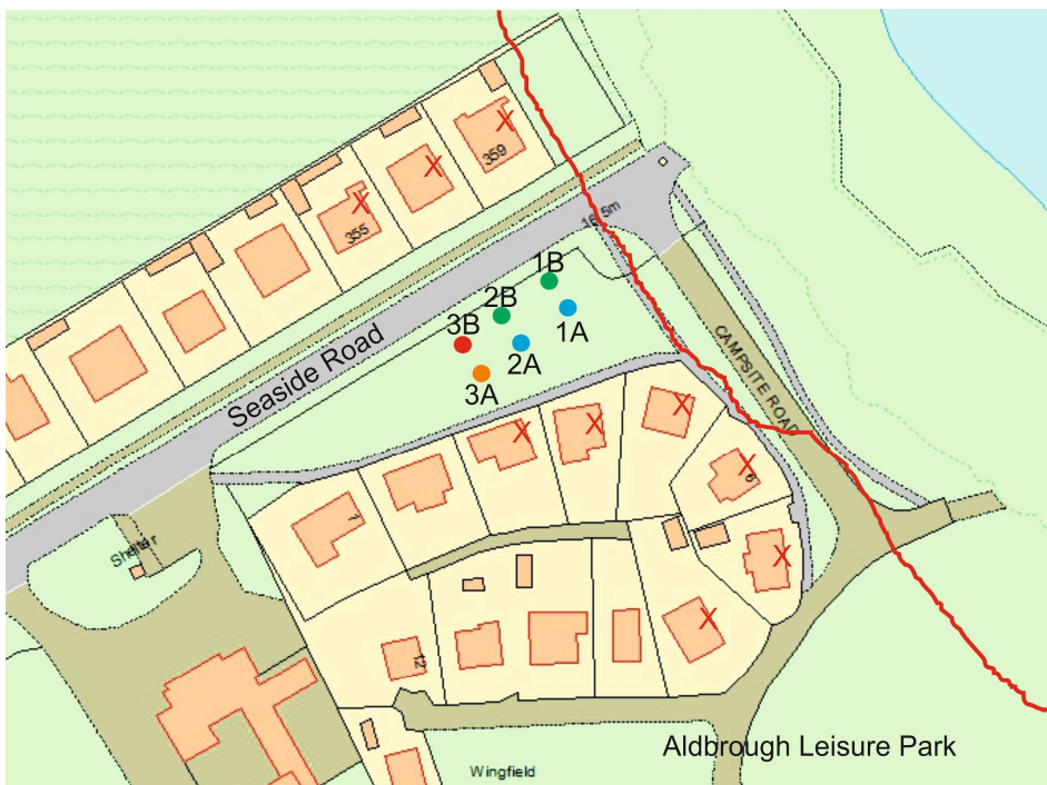
Figure 2 Approximate location of BGS boreholes NOTE: approximate cliff-top position (red line) as at 2013. NOTE: Boreholes 1A, 1B, 2A & 2B drilled in March 2012, boreholes 3A & 3B drilled in January 2015. NOTE: Properties marked with X have been demolished (as at Jan 2015)
