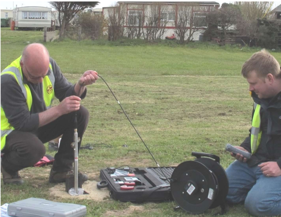
Figure 18 Borehole inclinometer monitoring - Insertion of inclinometer probe into borehole 1b (A- direction, landward)
