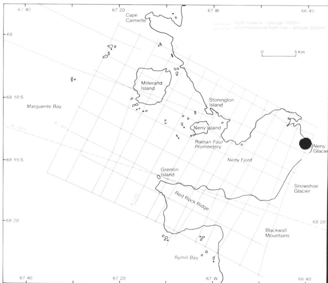
3(a) Fig. 3. Map of Neny Fjord area showing: (a) flight lines and (b) total-intensity magnetic anomalies. Contour interval 50 nT, bolder contours every 250 nT. Flight altitude 1000 m.
