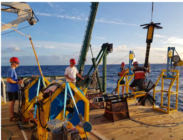
Figure 4: Back deck of the RV Walton Smith showing VMP winch/line puller setup.
