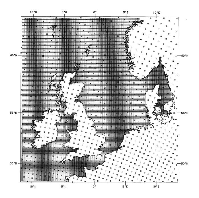
Figure 1. CS3 model grid with LAM atmospheric model points.
