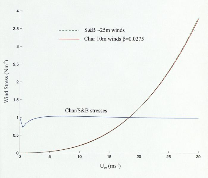
Figure 3. Variation of surface stress with wind speed. Comparison of estimates using LAM with the Smith & Banke drag coefficient and MES 10m winds with Charnock. The ratio (blue line) is very close to 1.
