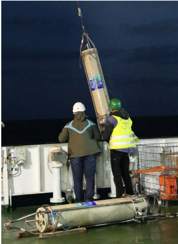
Fig. 5: Recovery of a marine snow catcher during the DY077 cruise. Another marine snow catcher is seen lying on deck. After placing the marine snow catcher upright for a period of time, the aggregates will settle out and can be collected from the lower, detachable part of the marine snow catcher.
