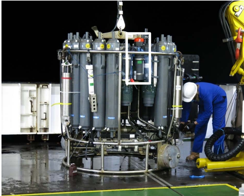
Figure 9 - Pre-deployment calibration CTD with Seaguard in place of one of the 20 L Niskin bottles, please note the Turner Cyclops fluorometer mounted on the top bar facing upwards out of the CTD rosette.
