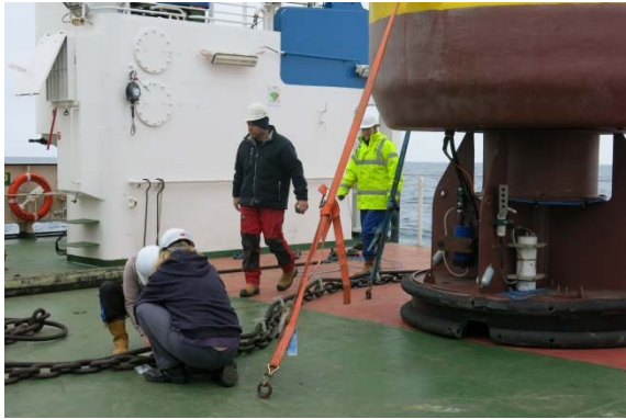
Figure 2: Buoy-to-Hub cable inside hydraulic hose clamped to mooring chain. At the bottom you can see the buoy with copper paint.
