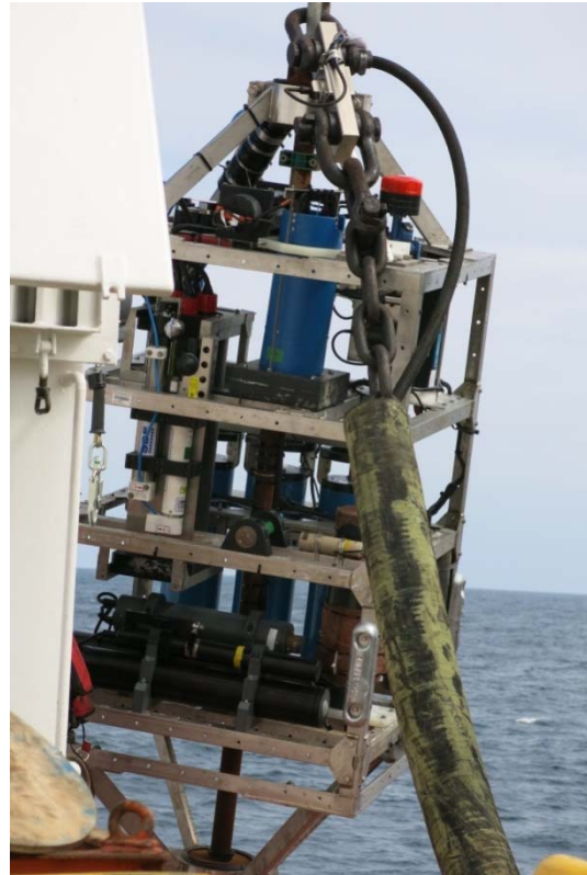
Figure 3: Sensor frame being deployed showing large hydraulic hose over mooring chain
