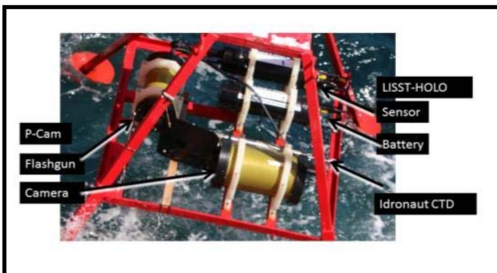
Fig. 2. The Red Camera Frame (RCF) with the PELAGRA Cam and the LISST HOLO (Holocam).
