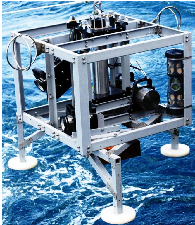
Bathysnap DY077-084 as deployed, note 4 larval traps top centre of frame around release position, and tube of colonisation substrata on the rear upright on the flash side.
