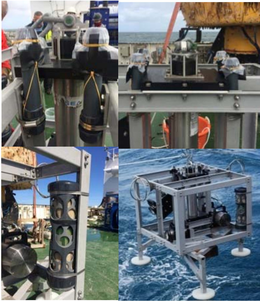
Figure 57. Bathysnap with one LO 3 CAted settlement frame attached upright on the rear of flash side and four larval traps attached on the top centre of the frame around release.
