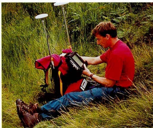
Using GPS and pen-computer technology to collect map data during fieldwork, for the Countryside Survey 2000.
