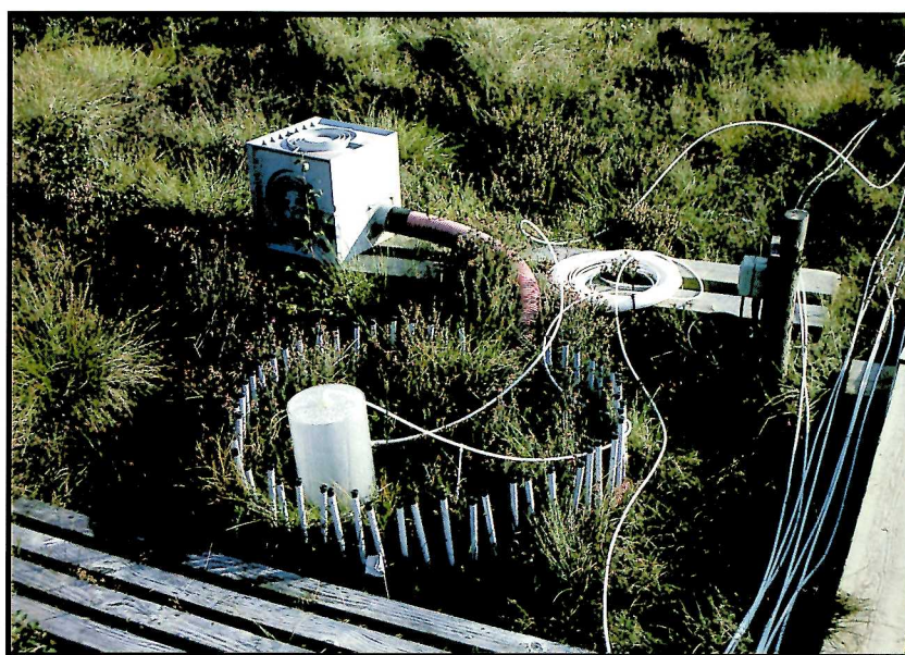
Plate 18. Equipment for maintaining a higher concentration of carbon dioxide in the air over a small plant community. The large difference in \delta^{13}\text{C} signature between the added \text{CO}_2 ( -44\text{‰} ) and ambient ( -8\text{‰} ) allows measurement of incorporation of ^{13}\text{C} into the community
