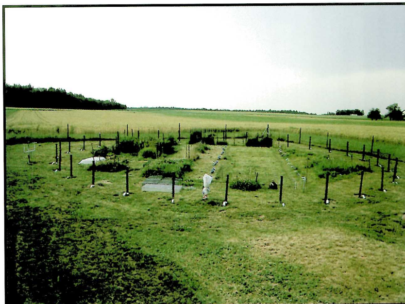
Plate 17. FACE experimental plot at ETH, Zurich, showing the ring of CO 2 release pipes
