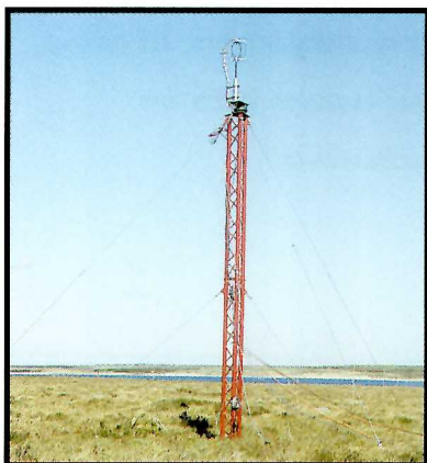
Plate 18. Measuring carbon dioxide fluxes over undisturbed Scottish peatland
