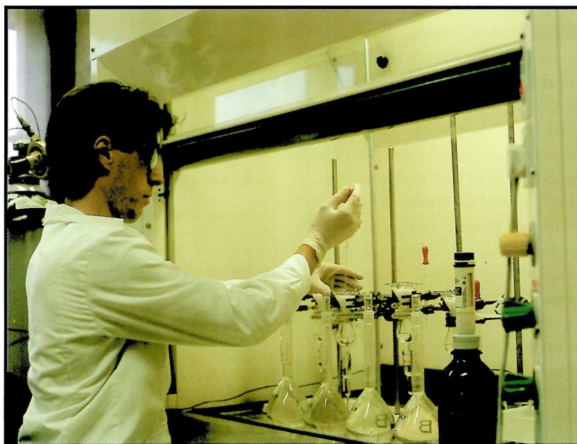
Plate 20. Preparation of river water samples for analysis by GC-MS and GC-ECD
