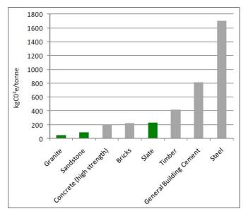
Figure 5 Embodied carbon in common construction materials (from SFGB, 2011)
