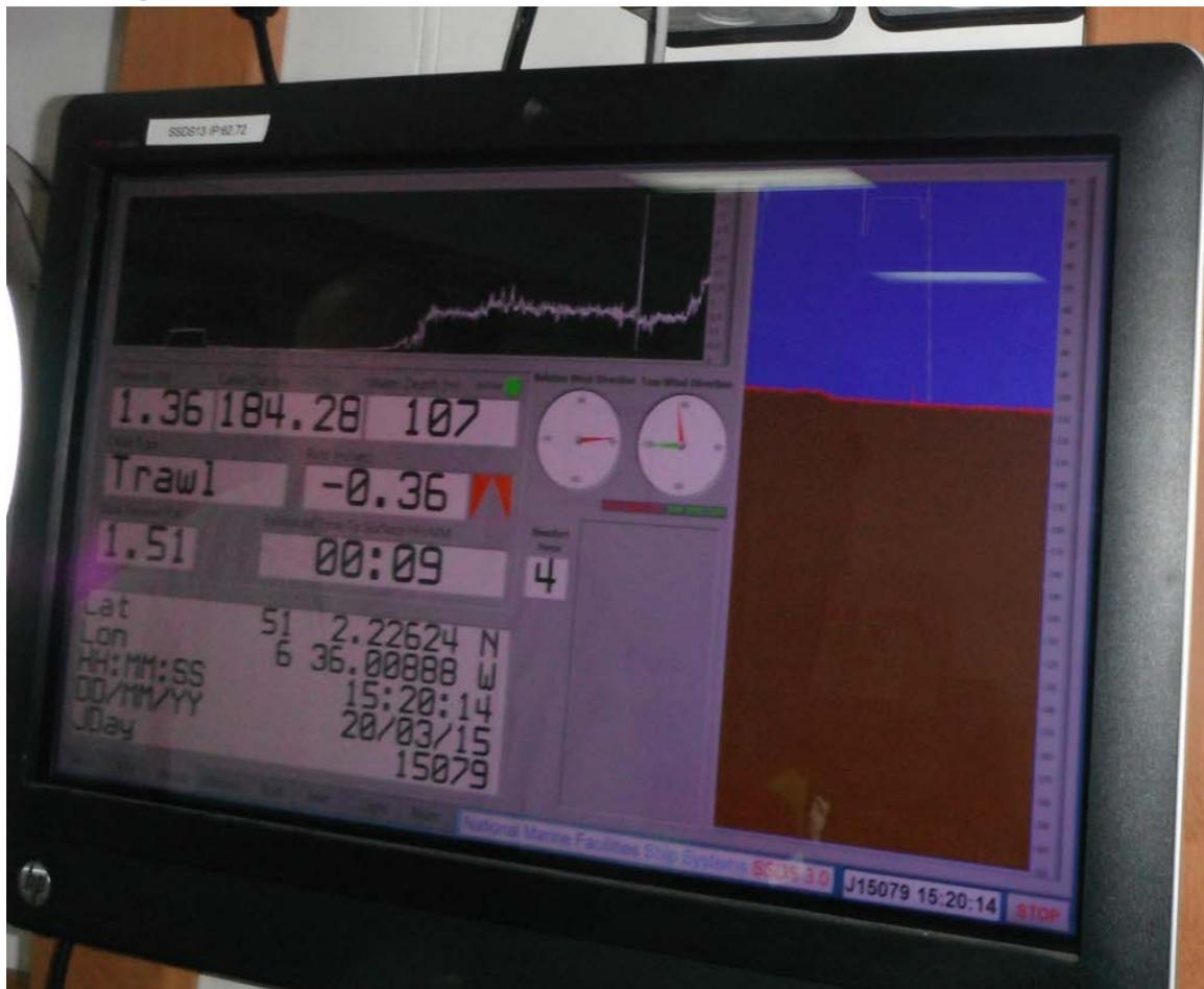
**Fig. B8. Monitoring of the ships position, the trawl line length and the trawl line tension**
