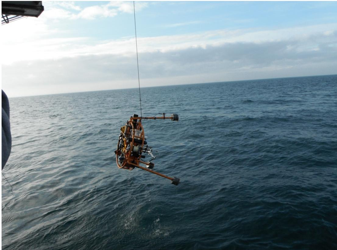
**Fig. B10. Recovery of the lander with the ground line wrapped around one of the larger battery cases that protruded from the lander frame**
