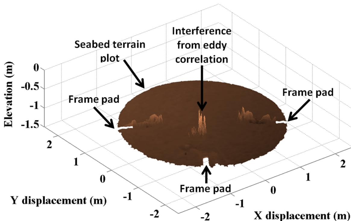
**Fig. 11. Preliminary plot of the seabed terrain using the 3D ripple profiling sonar**
