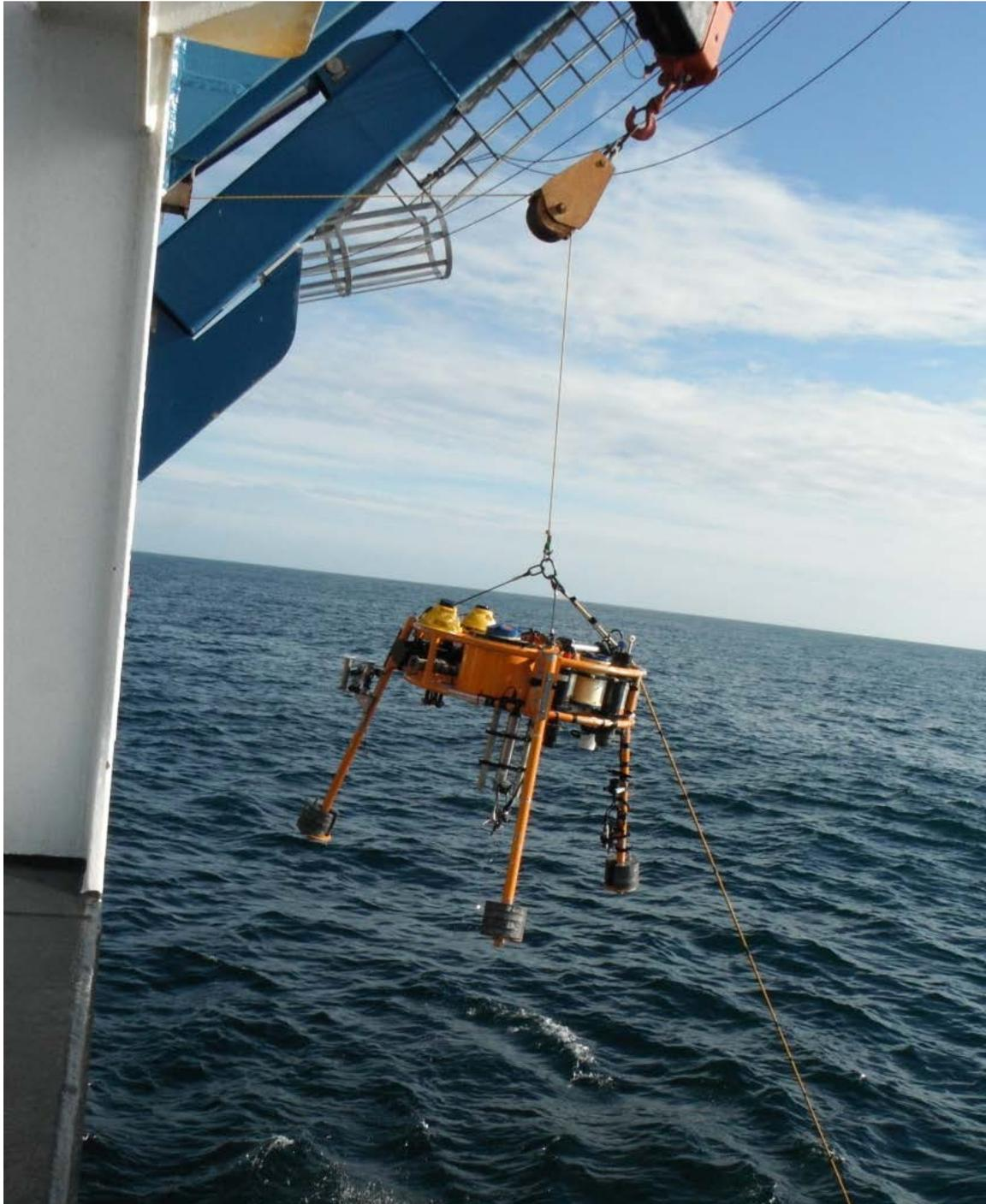
**Fig. B16. Recovery of the miniSTABLE frame with the mooring ground line still attached**
