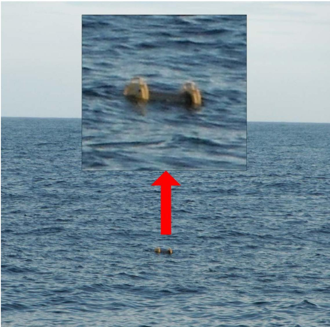
**Fig. B15. Backup recovery float on the surface with the 250m frame to float line fully deployed**
