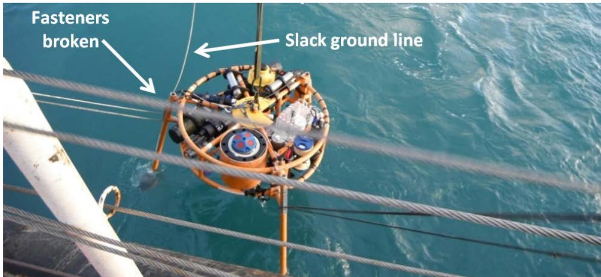
**Fig. C2.** The plastic fastenings of the ground line along one of the frame legs was broken
