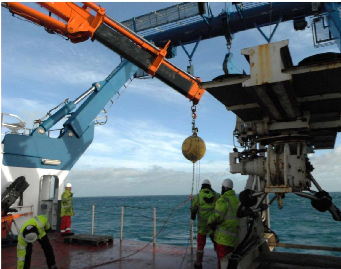
**Fig. B5. miniSTABLE frame deployment over the stern of RRS Discovery**
