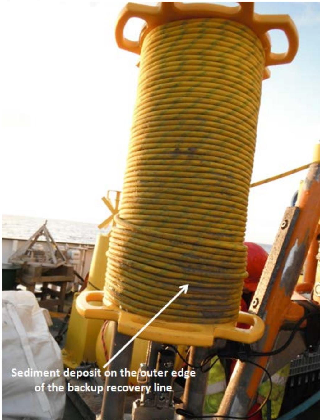
**Fig. C8. Sediment build up on the outer edge of the recovery spooler indicating the frame tipping had occurred during the lander frame recovery**
