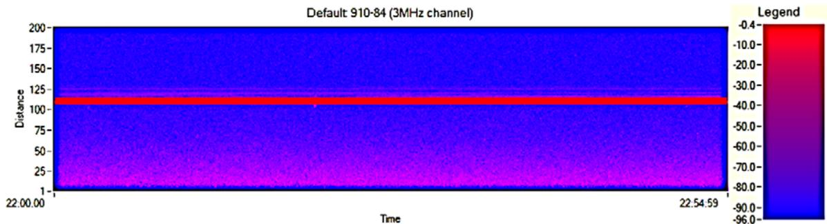
**Fig. 22. Plot of 3MHz reflected signal strength from 1 hour of data at the benthic H survey site**
