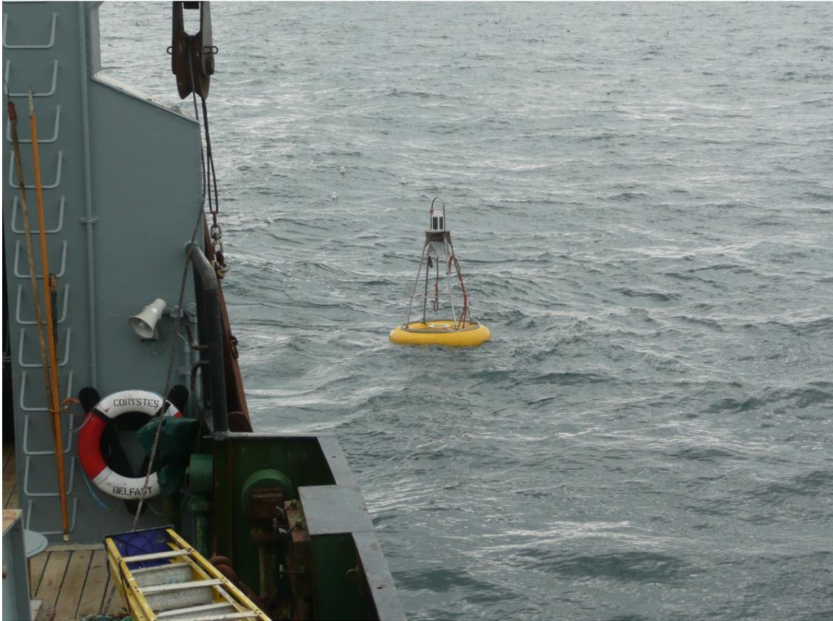
**Fig. B19. Possible alternative surface expression for a lander frame L shaped mooring**
