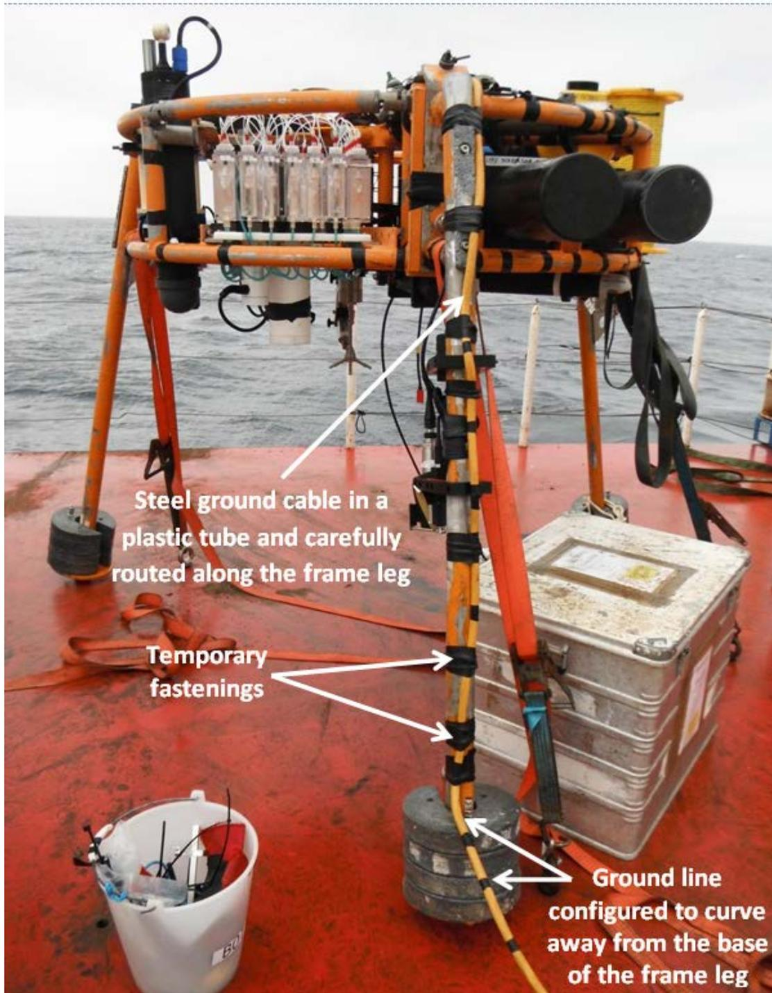
**Fig. C4.** A yellow plastic tube used for ground line steel cable insulation as shown in the picture. The fastening points along one of the frame legs and the curvature of the ground line away from the frame, as used during the DY034 research cruise, can be seen.
