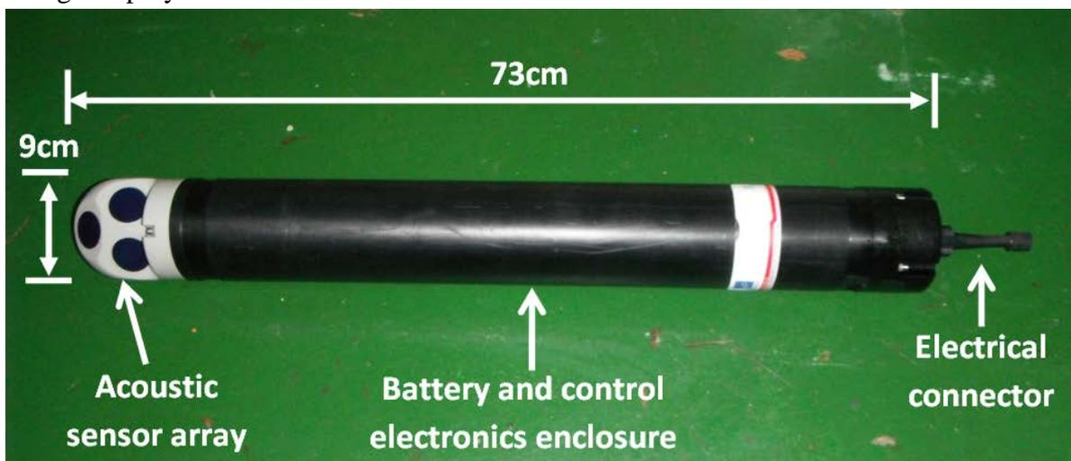
**Fig. 18. The Nortek Aquadopp HR was used as a downward facing water velocity sensor**
