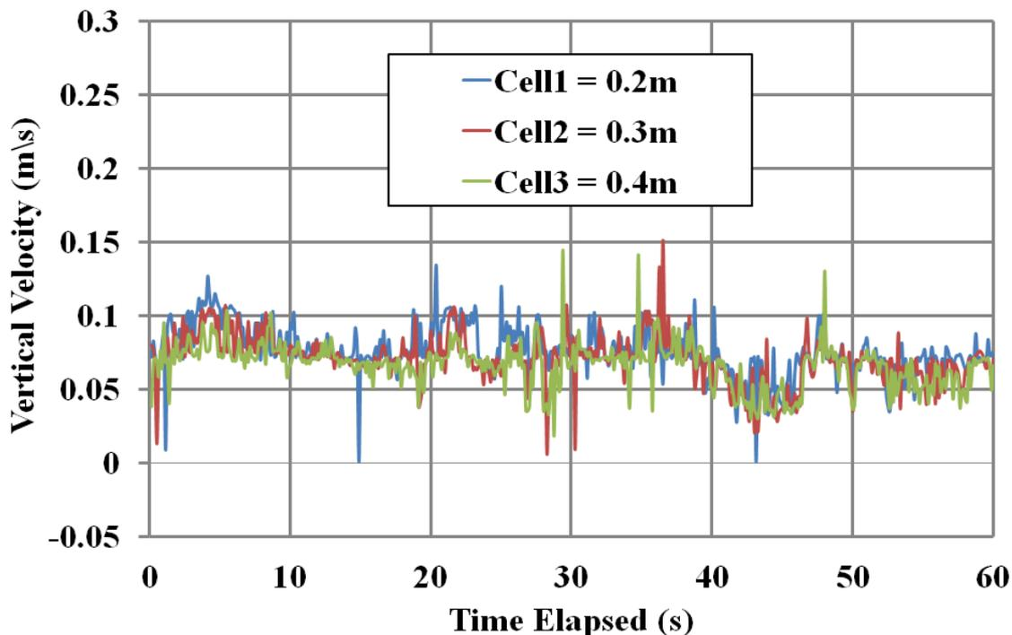
**Fig. 19. Plot of velocity profiles from the Aquadopp HR from a deployment at the benthic A survey site during the DY34 research cruise**
