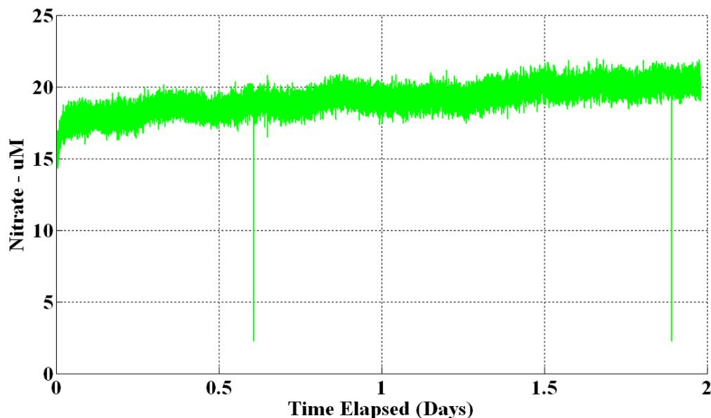
**Fig. 13. Example Plot of Satlantic SUNA measured output**
