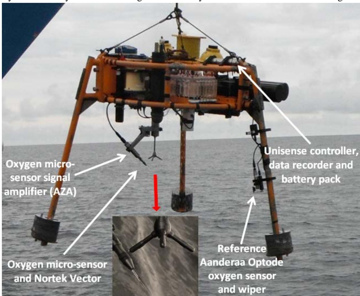
Fig. 27. The Unisense version 1 Eddy Correlation system with dissolved oxygen micro-sensor, reference Aanderaa Optode dissolved oxygen sensor and a Nortek Vector underwater velocity meter
