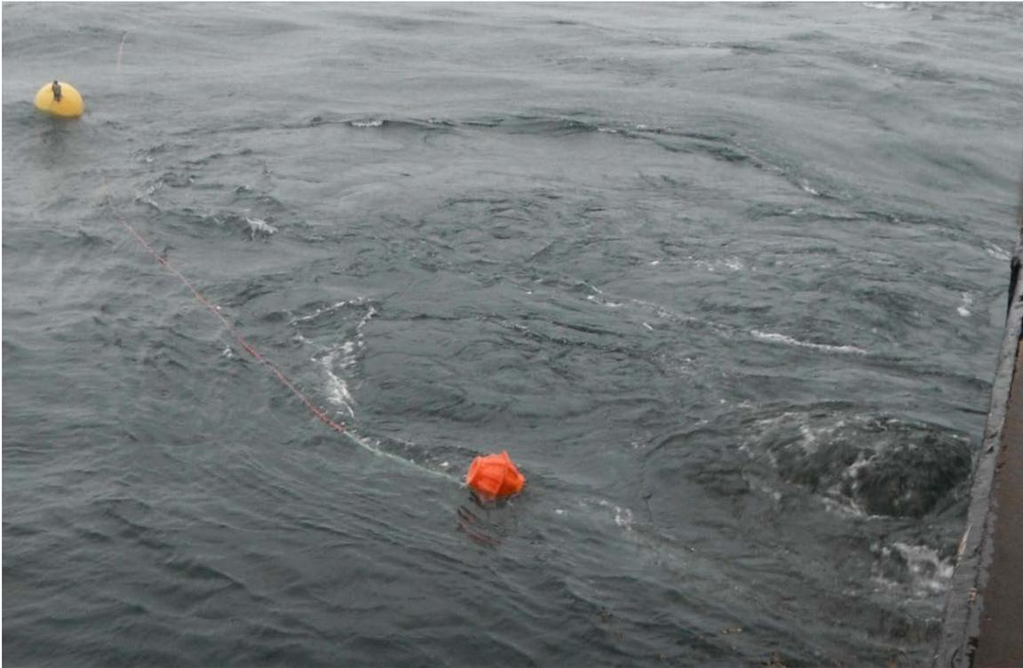
**Fig. B6. Deployed surface buoy and recovery float**
