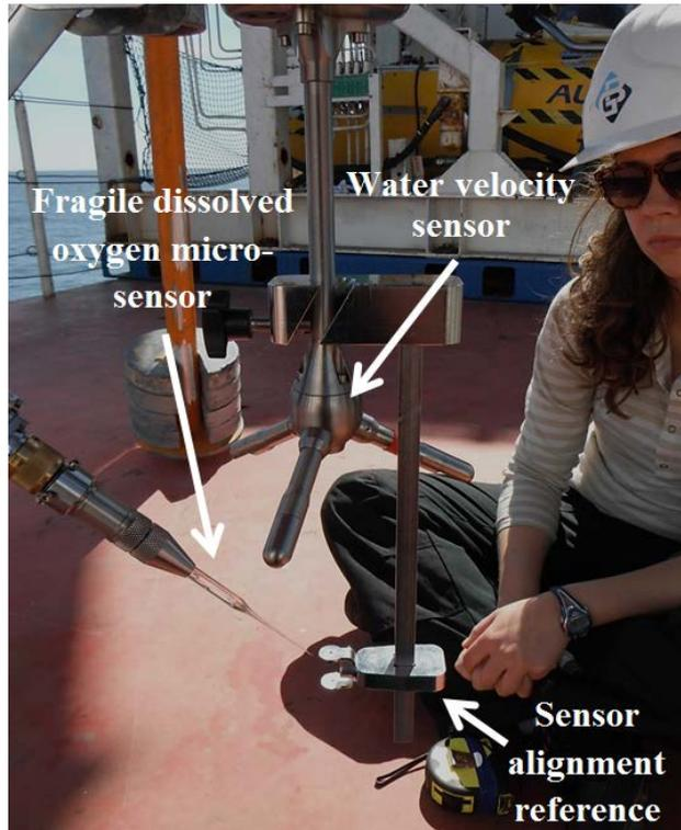
**Fig. B2.** Setup and alignment of the eddy correlation sensors underneath the miniSTABLE frame
