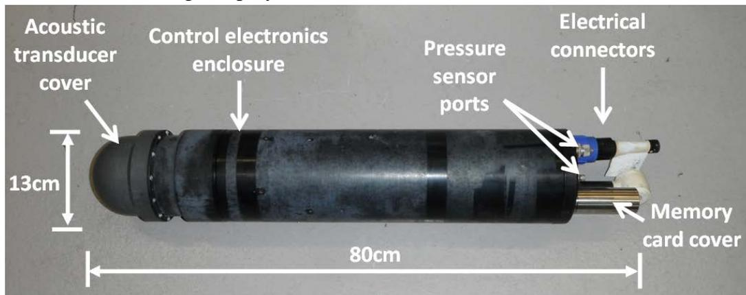
**Fig. 10. The 3D Sand Ripple Profiling and Logging Sonar**
