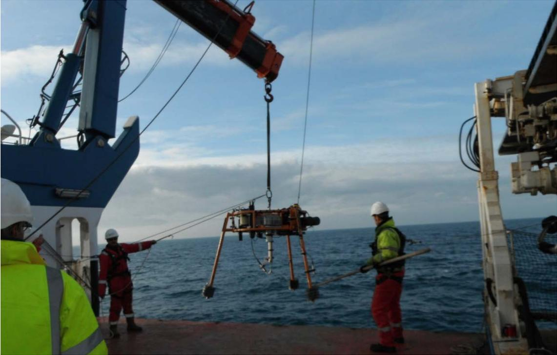
**Fig. B11. A Crane, strop, stay line and boat hook used to re-orientate the frame during the recovery**
