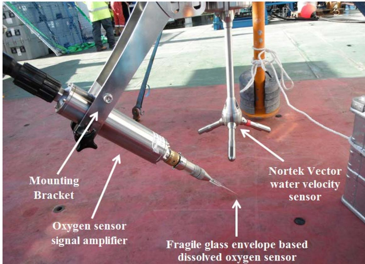
**Fig. 4. The eddy correlation sensing arrangement**
