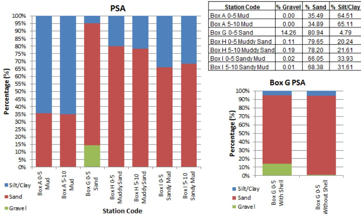
**Fig. A3. The Benthic A, G, I and H survey site sediment Particle Size Analysis (PSA)**
