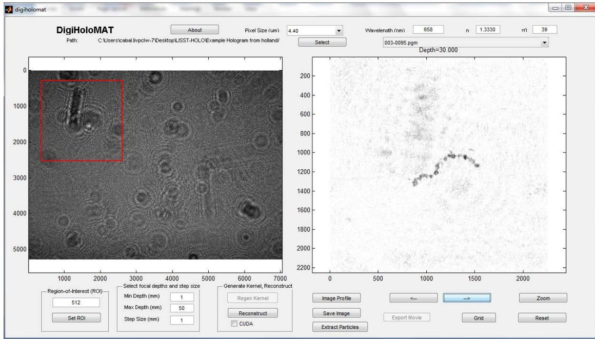
**Fig. 9. RRS Discovery DY030 research cruise LISST-HOLO raw composite image and region of interest image slice at a depth of 30mm into the sample volume. The scale is in  $\mu\text{m}$ .**
