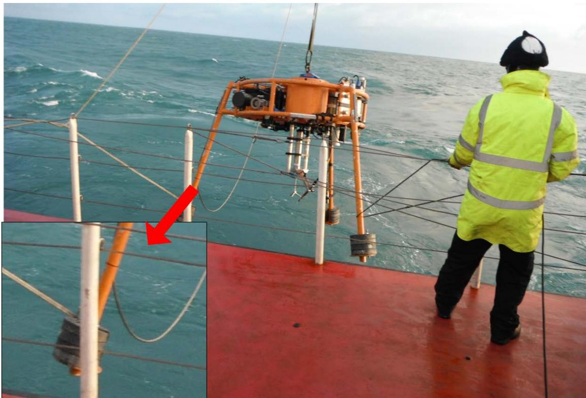
Fig. C1. A temporary plastic fasteners were used to keep the ground line cable in position along a preferred route from the central lifting coupling along the lander frame and down one of the frame legs
