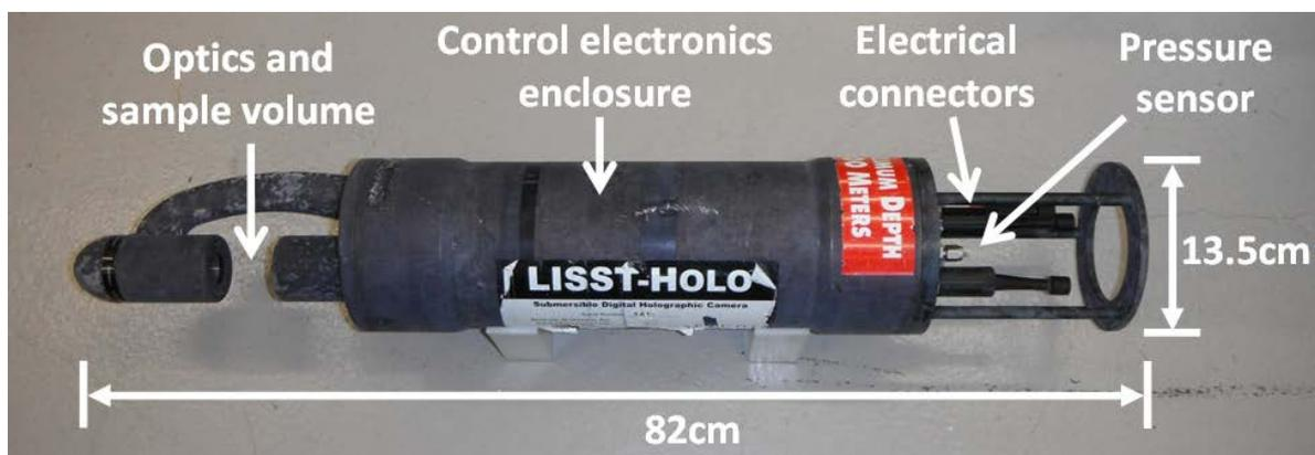
Fig. 8. The Sequoia LISST-HOLO holographic particle size analyser
