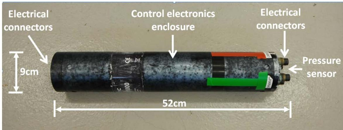
**Fig. 20. Basic layout of the Aquatec Aquascats 1000r**
