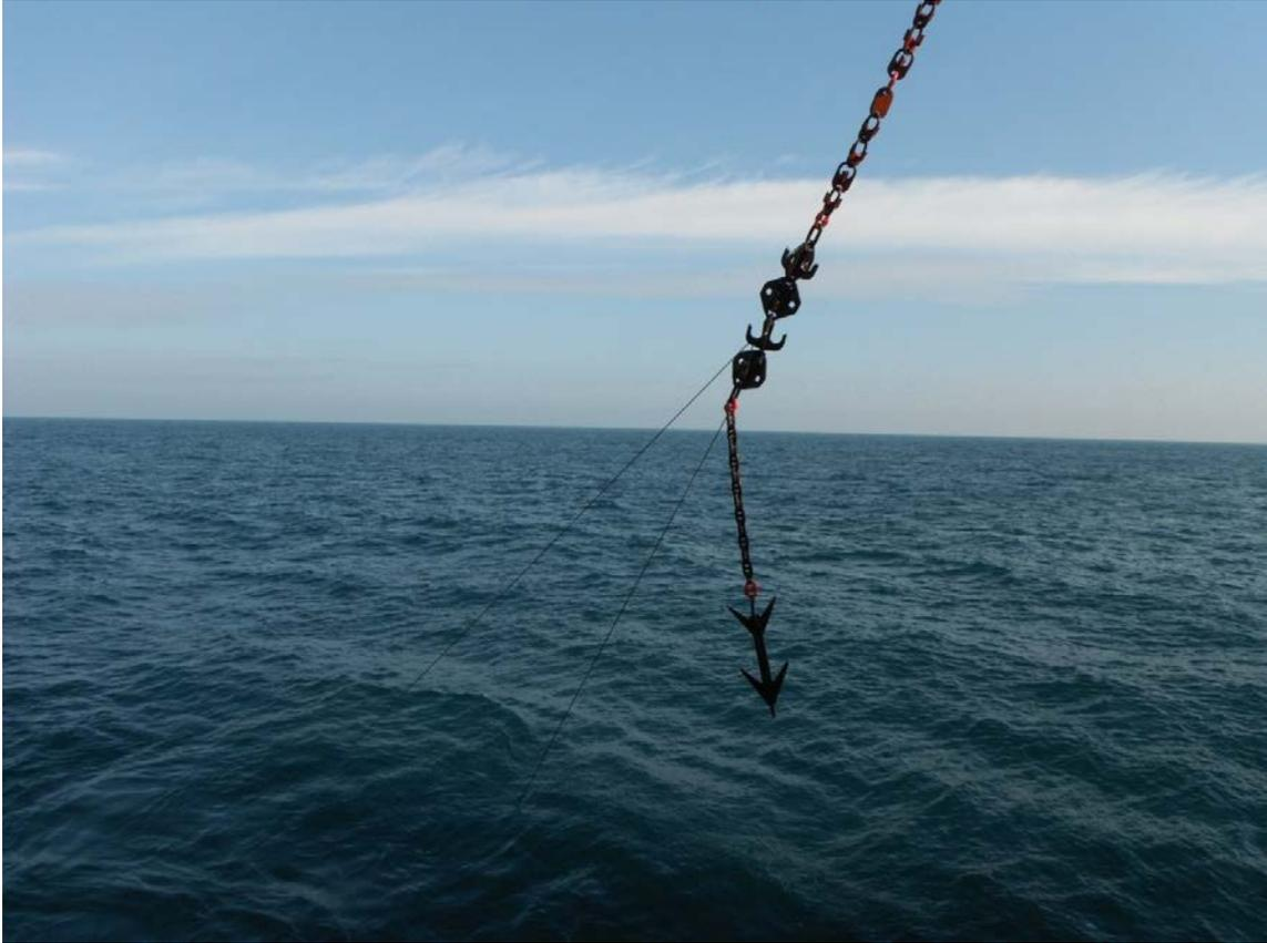
**Fig. B9. Recovery of trawl equipment with the miniSTABLE to cast anchor ground line snagged**
