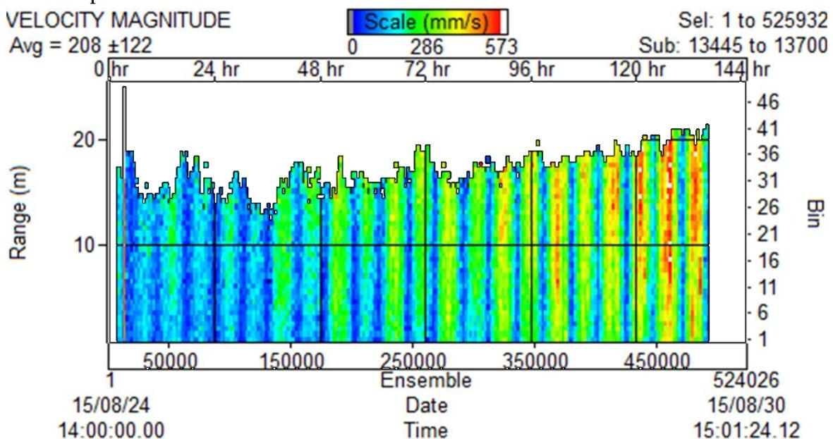
**Fig. 24. Plot of velocity profiles measured by the ADCP during a DY034 deployment**
