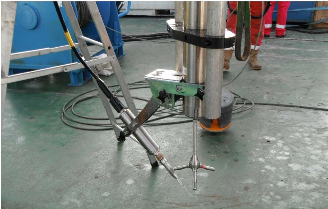
**Fig. B12. The glass oxygen micro-sensor and Nortek Vector from the eddy correlation system underneath the frame were still intact after the trawl recovery**
