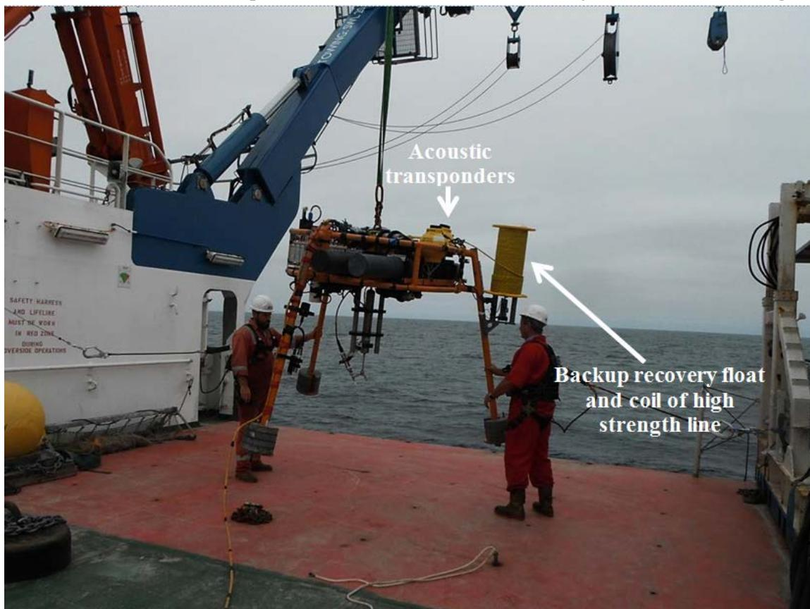
**Fig. B14. Deployment of miniSTABLE benthic lander frame with a float and a spool of high strength line to form a backup recovery system**
