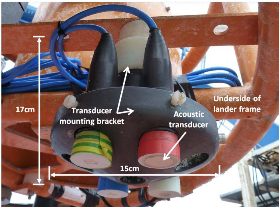
**Fig. 21. Close up picture of Aquascats 1, 2, 3 and 4 MHz transducers and mounting**
