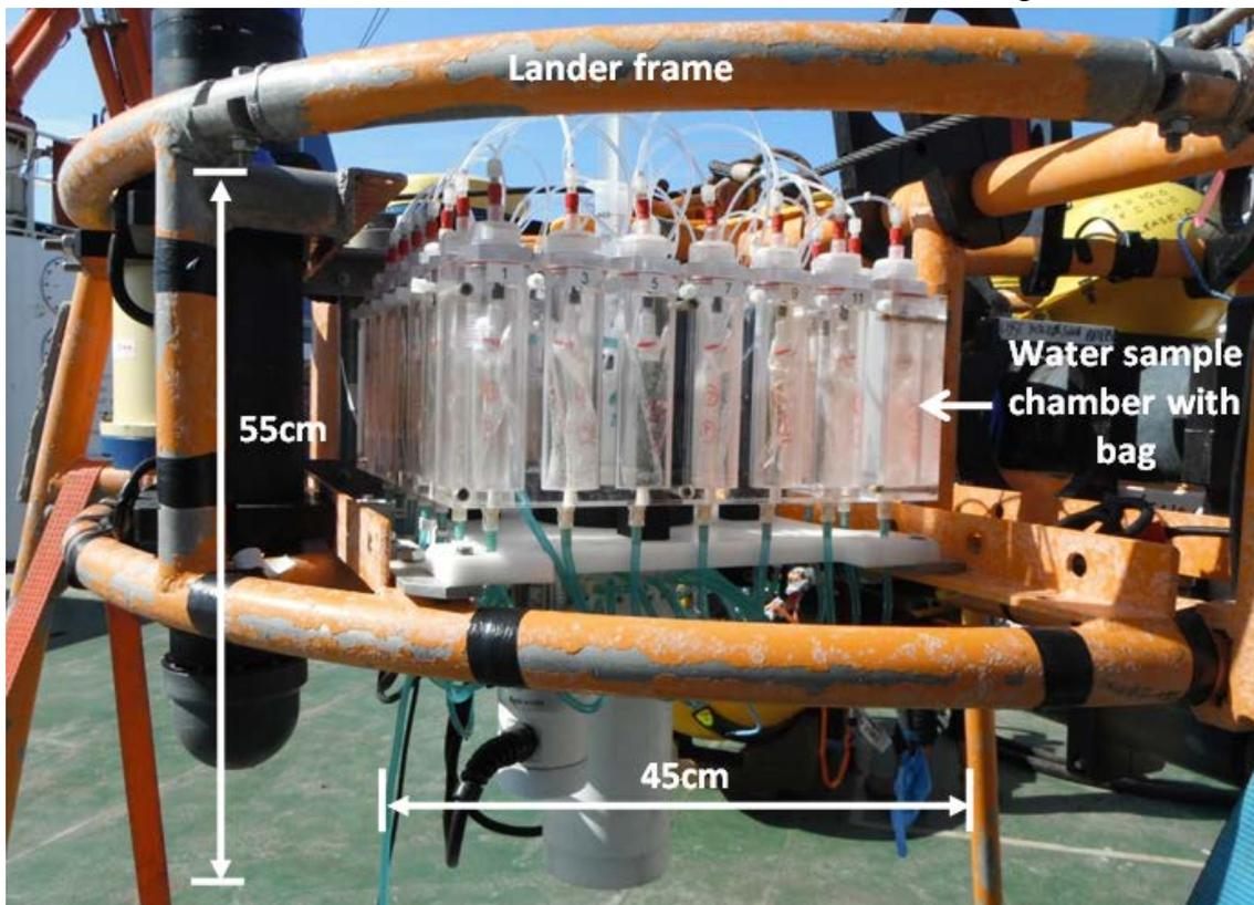
**Fig. 25. McLane RAS100 water sampler mounted on the NOCL seabed based lander frame**
