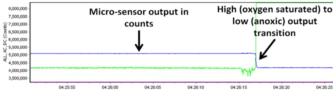
**Fig. 28. The Eddy correlation system micro-sensor probe response during the DY030 research cruise**
