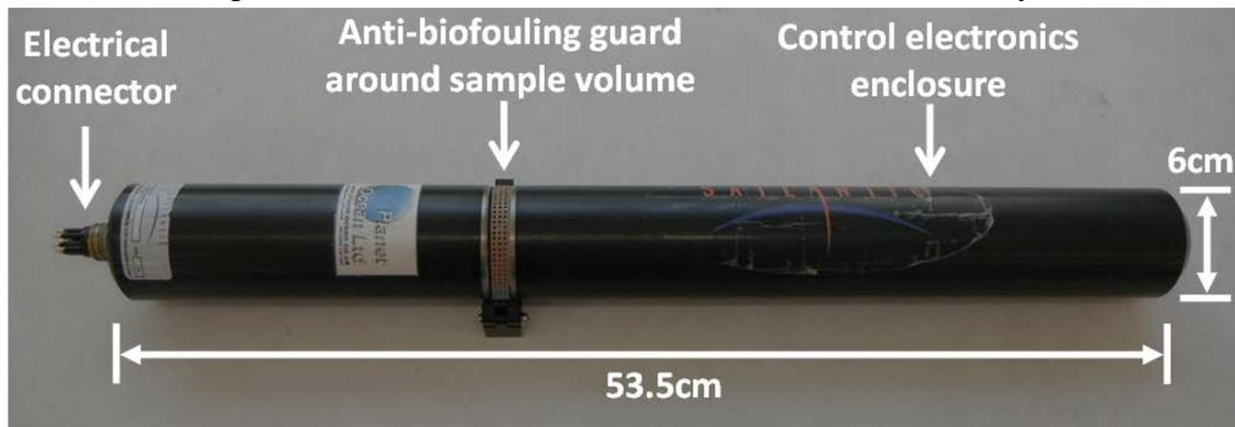
**Fig. 12. The Satlantic SUNA optical nutrient sensor**
