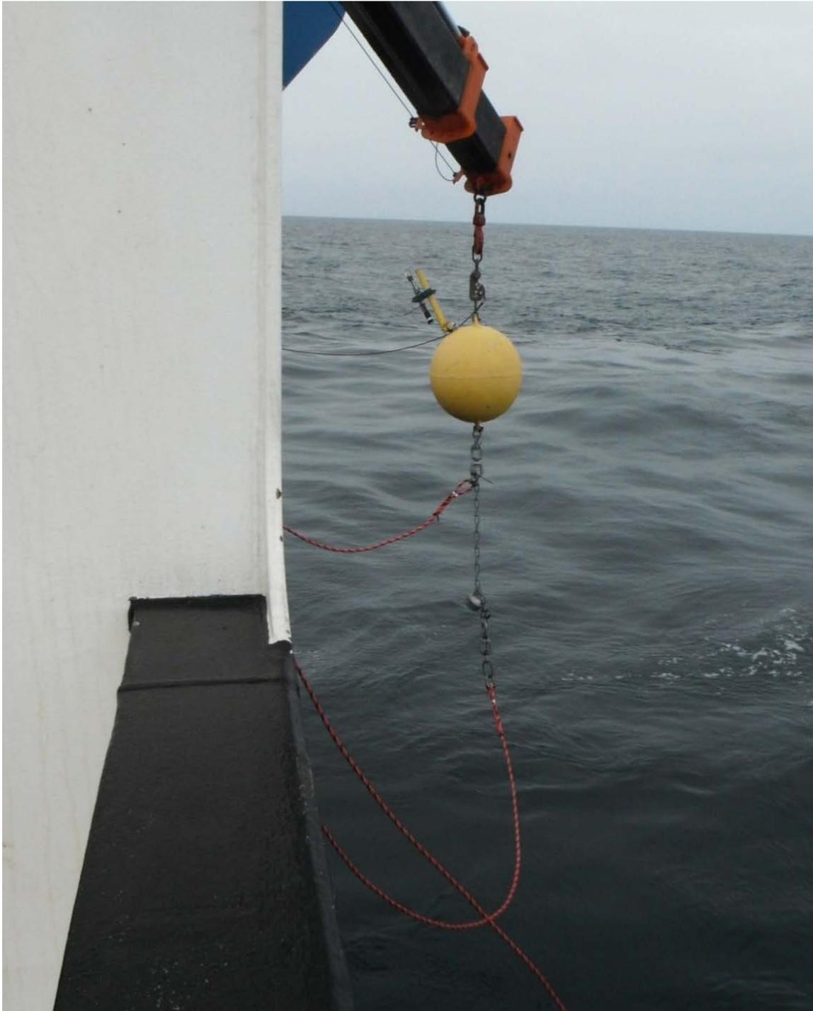
**Fig. B18. Modified mooring arrangement used during the DY030 research cruise to discourage recovery line entanglement via an underside chain and double swivel link coupling**
