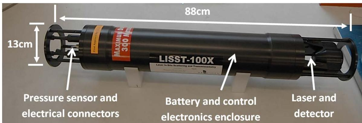
Fig. 6. The Sequoia LISST-100X laser in-situ transmissometry
