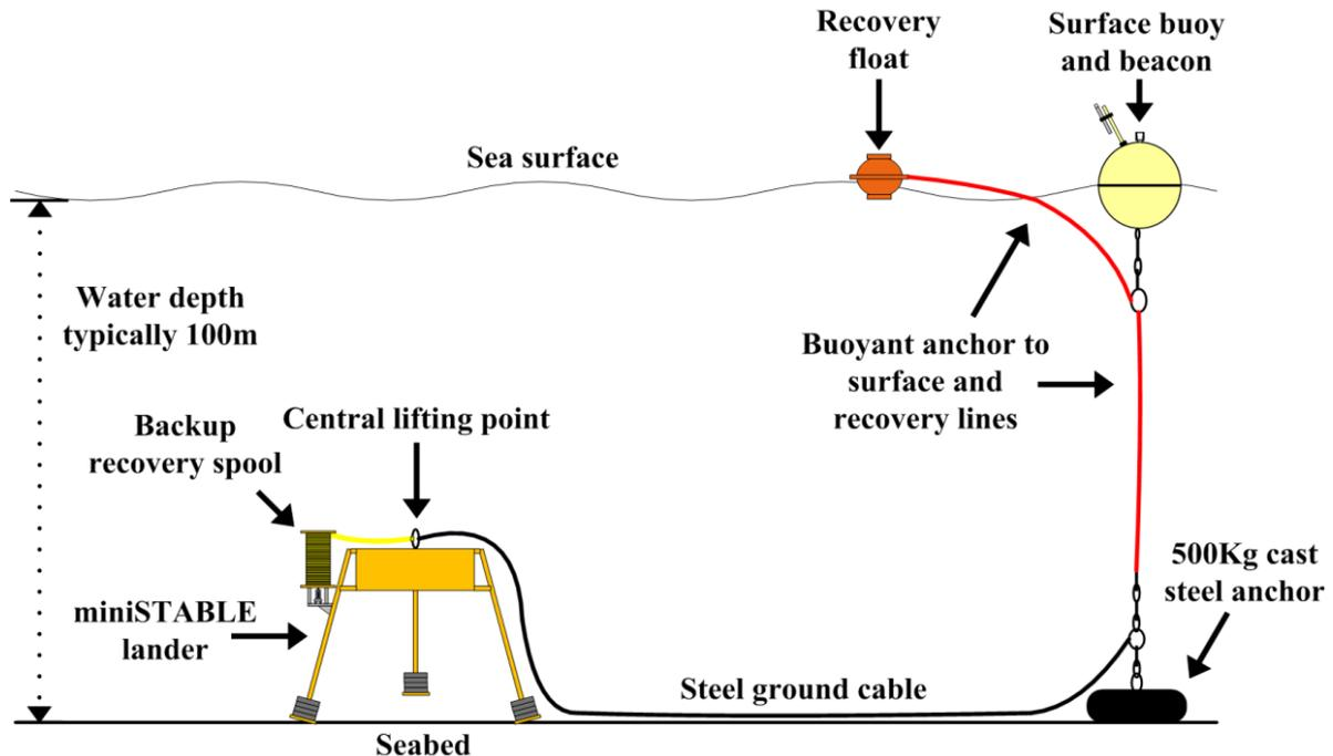
**Fig. 3. Simplified mooring functional diagram**
