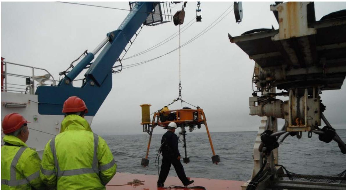
**Fig. C7. Lander frame recovery using the triple line frame lifting harness during DY034**
