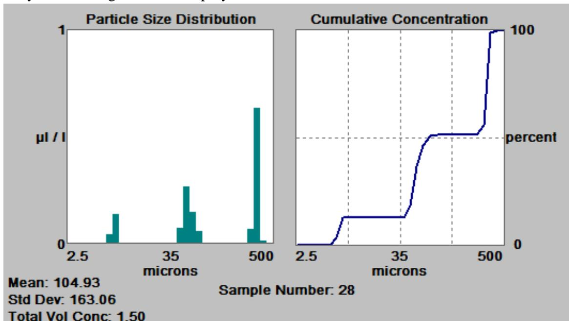
Fig. 7. LISST-100X particle size distribution plot using the manufacturers software
