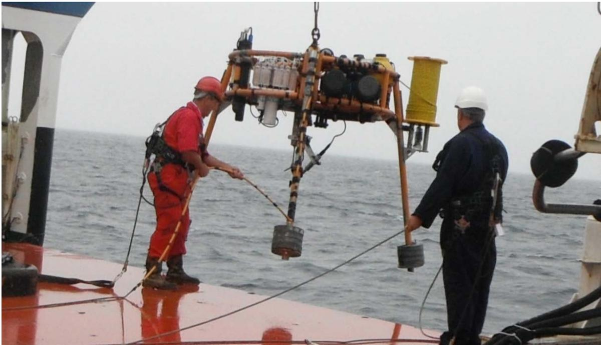
**Fig. C5. Use of the ground line fastened to one of the frame legs to control the lander frame position and dampen any frame oscillations during a DY034 research cruise deployment**
