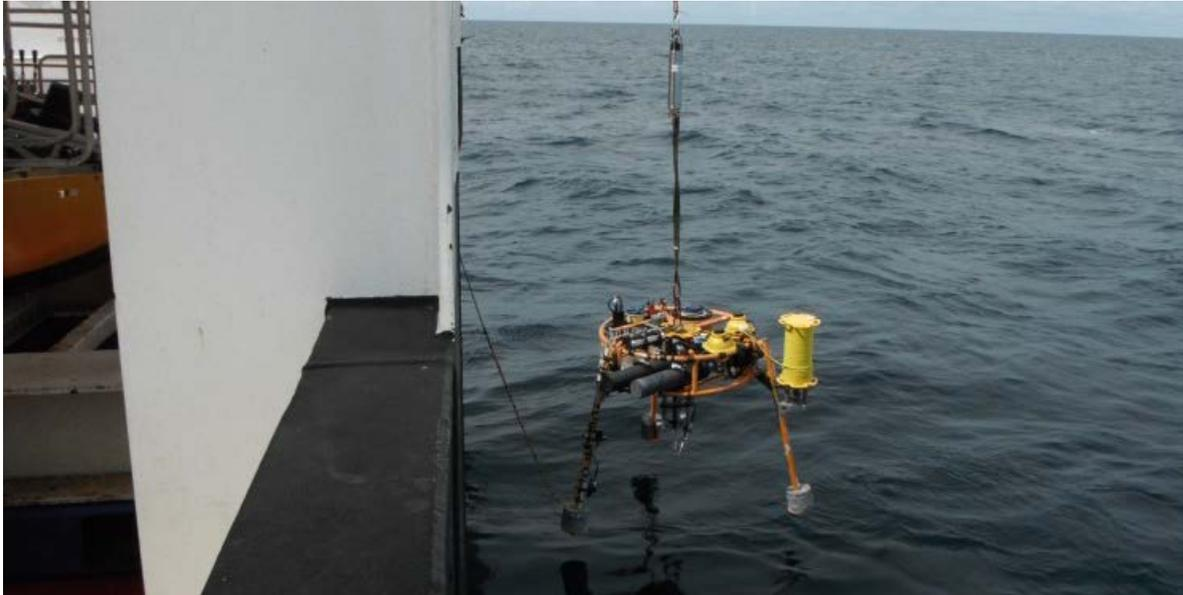
**Fig. C6. Limited ground line tension was used to control the frame alignment during the critical initial phases of a deployment during DY034.**
