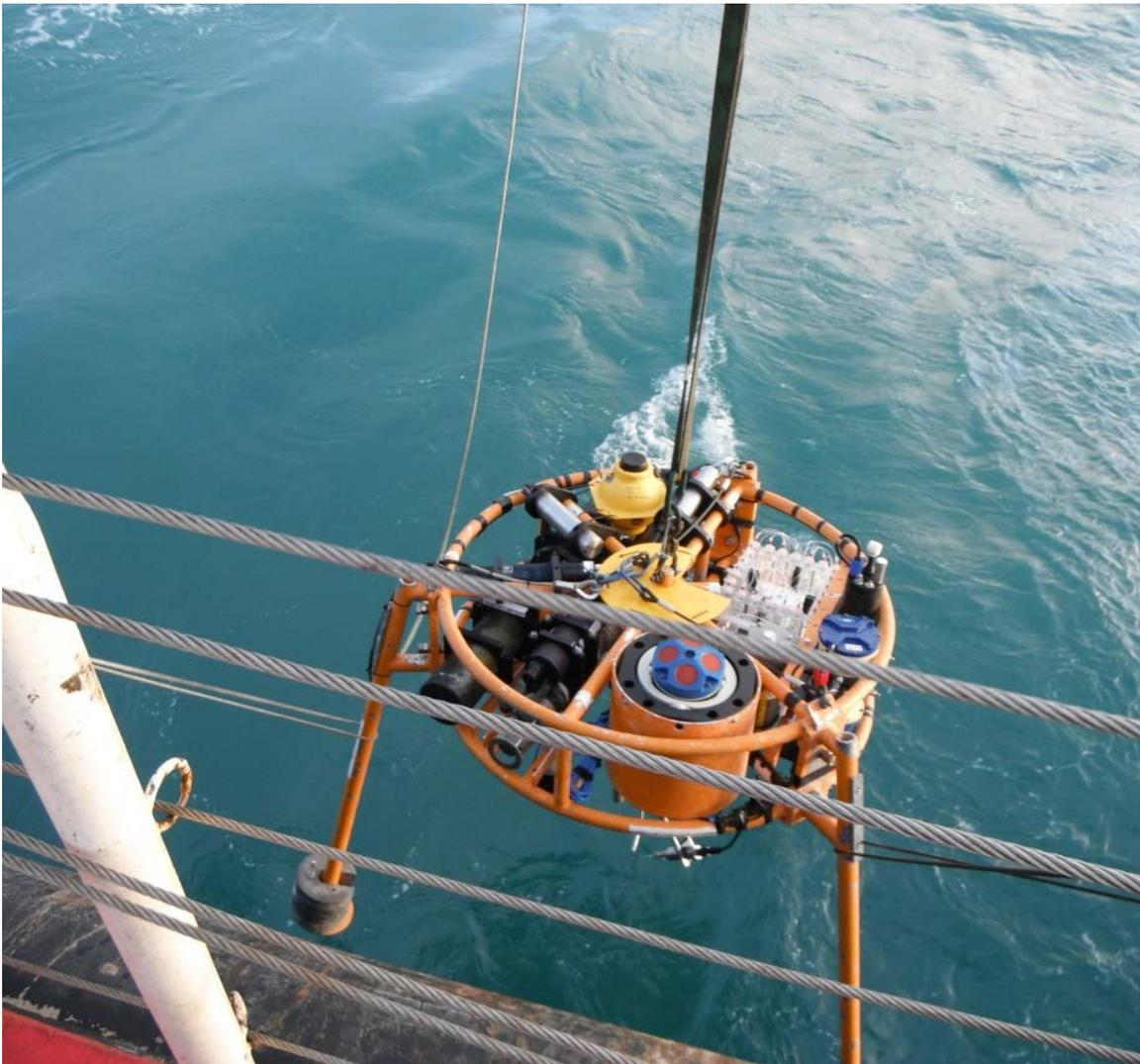
**Fig. B4. miniSTABLE frame deployment over the stern of RRS Discovery**
