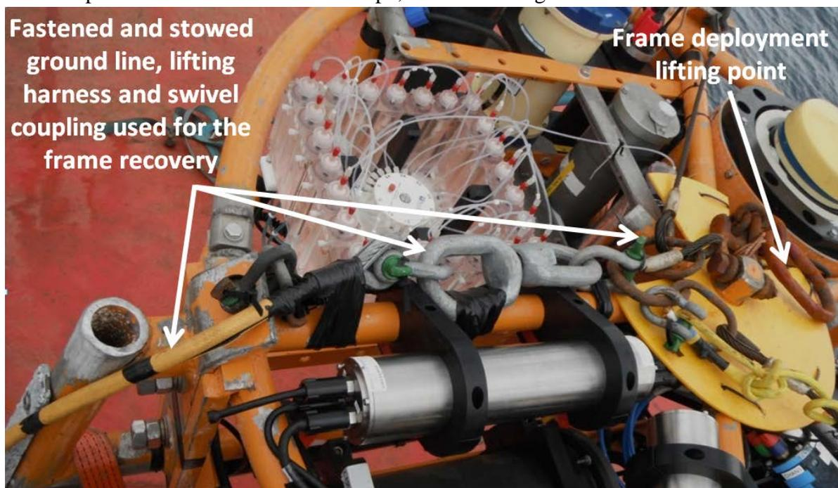
**Fig. C3.** Ground line fastening along the upper part of the frame, as used during DY034
