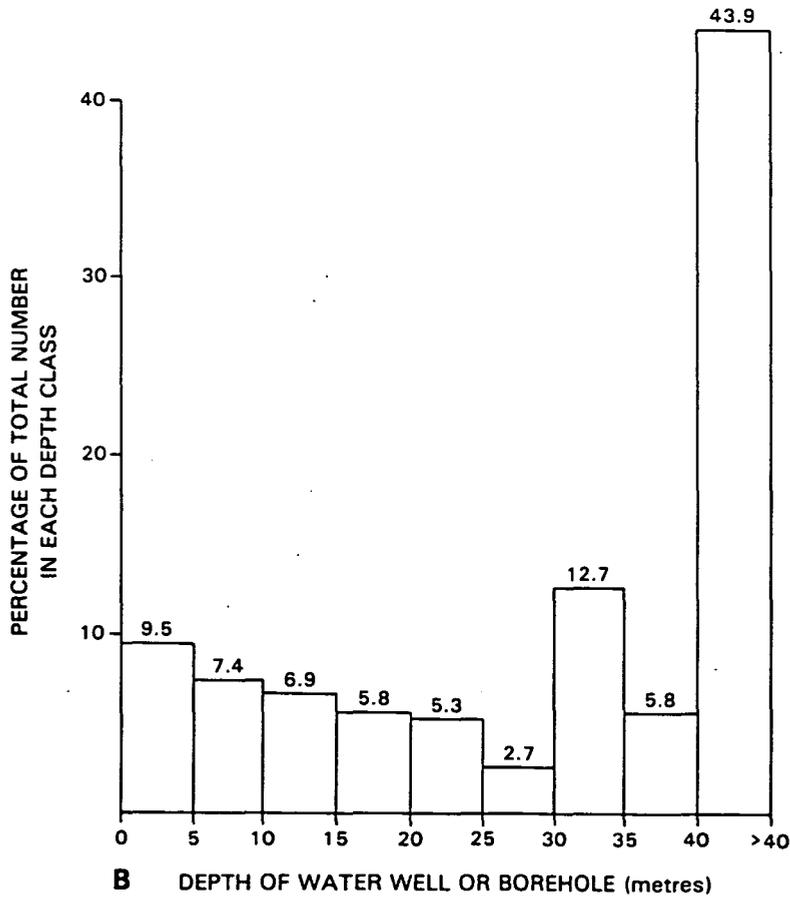
Figure 4. Histograms showing the distribution of the different depths to which A site investigation boreholes and trial pits and B water wells and boreholes have been sunk
