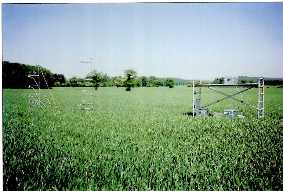
Plate 27. Micrometeorological instrumentation for determining \text{NH}_3 and \text{SO}_2 fluxes over a wheat canopy at the field site
