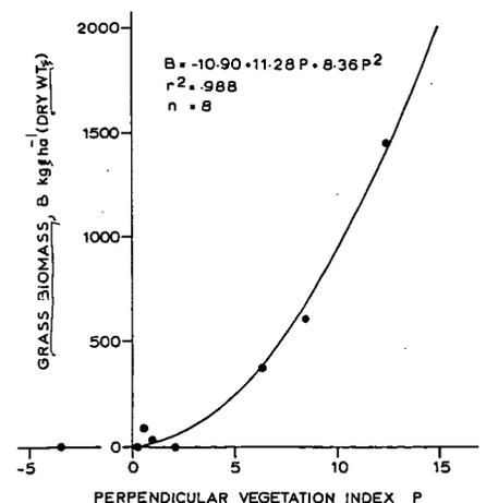
Figure 20. Calibration curve for prediction of dry grass biomass from the perpendicular vegetation index.
