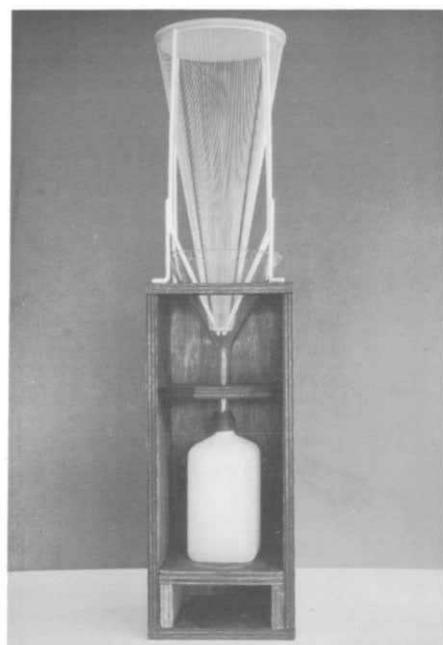
Figure 24. A fine filament gauge for collecting cloudwater droplets (see May, 1961) illustrates the construction of the open cloud gauge, with a polypropylene toothed edge lid, nylon collecting filaments, polyethylene coated frame, glass funnel and polypropylene collecting bottle.
