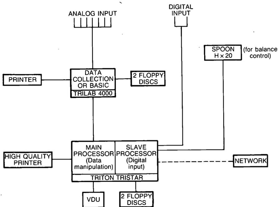
Figure 72. Plan of computerized laboratory system for analytical chemistry data
