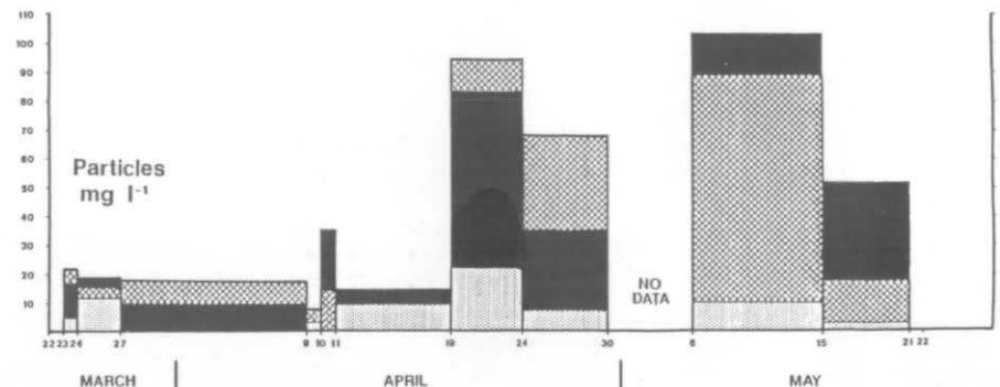
Figure 26. Histogram of particles ( $\mu\text{g l}^{-1}$ ) recorded for three gauge types, rainwater, open cloud gauge and lidded cloud gauge at Castlelaw Hill from 22nd March 1985 to 22nd May 1985. Each collection period spans between the sample dates untreated, producing time averaged concentrations.
