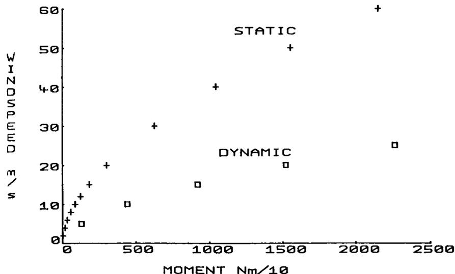
Figure 40. Bending moments under wind-loading measured at the base of a 12.4m tall Sitka spruce tree. The differing effects of wind applied constantly
