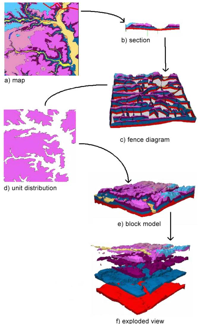
**Figure 1** The GSI3D workflow for modeling superficial and simple bedrock geology. The example covers the TM24 map area around Woodbridge in Suffolk and extends down to the top surface of the Chalk. The Lambeth Group is in red overlain by the London Clay in blue, the Red Crag in maroon, superficial sands and gravels in shades of pink and Loestoft Till (boulder clay) in pale blue.
