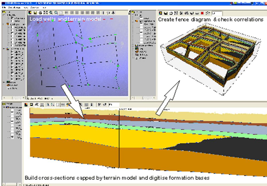
Figure 10 Fence diagram construction in GSI3D.
