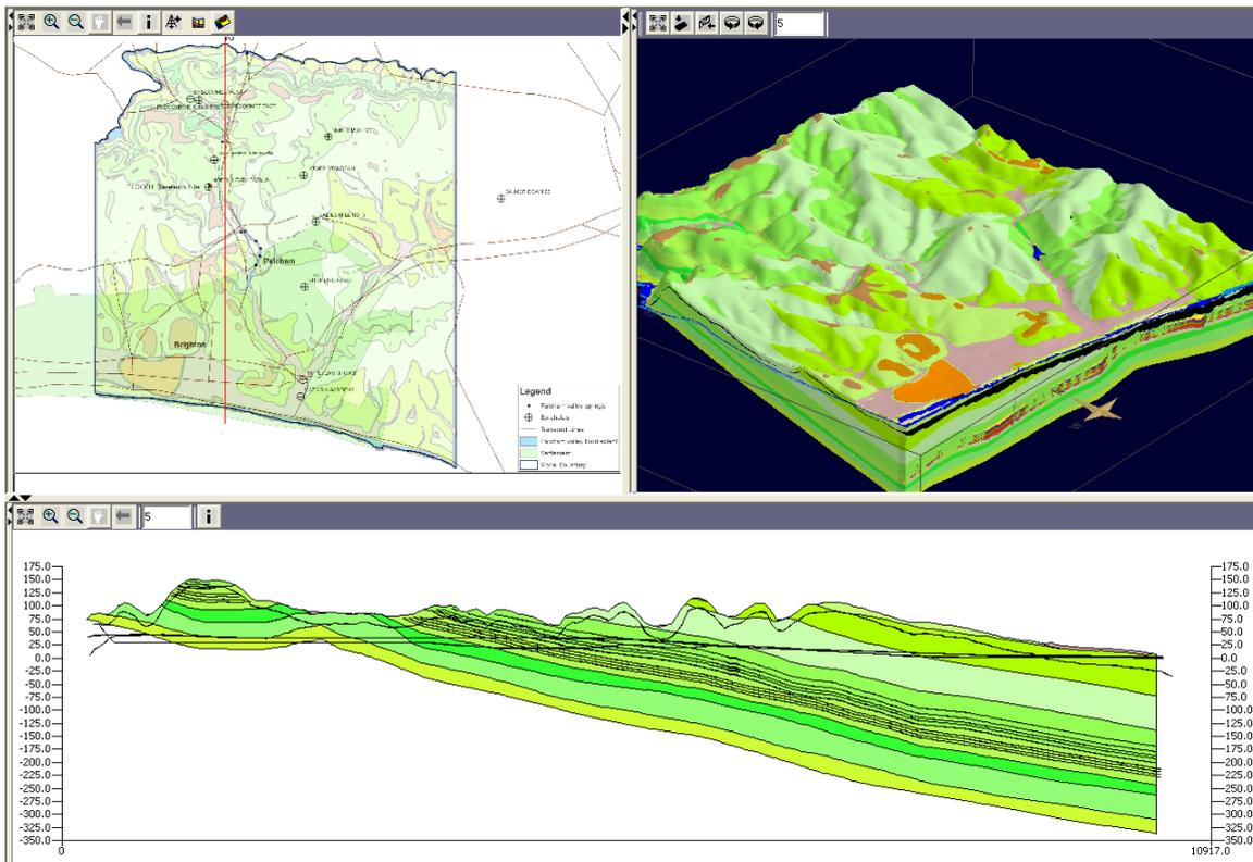
Figure 17 The Patcham 3D geological model in the subsurface viewer.
