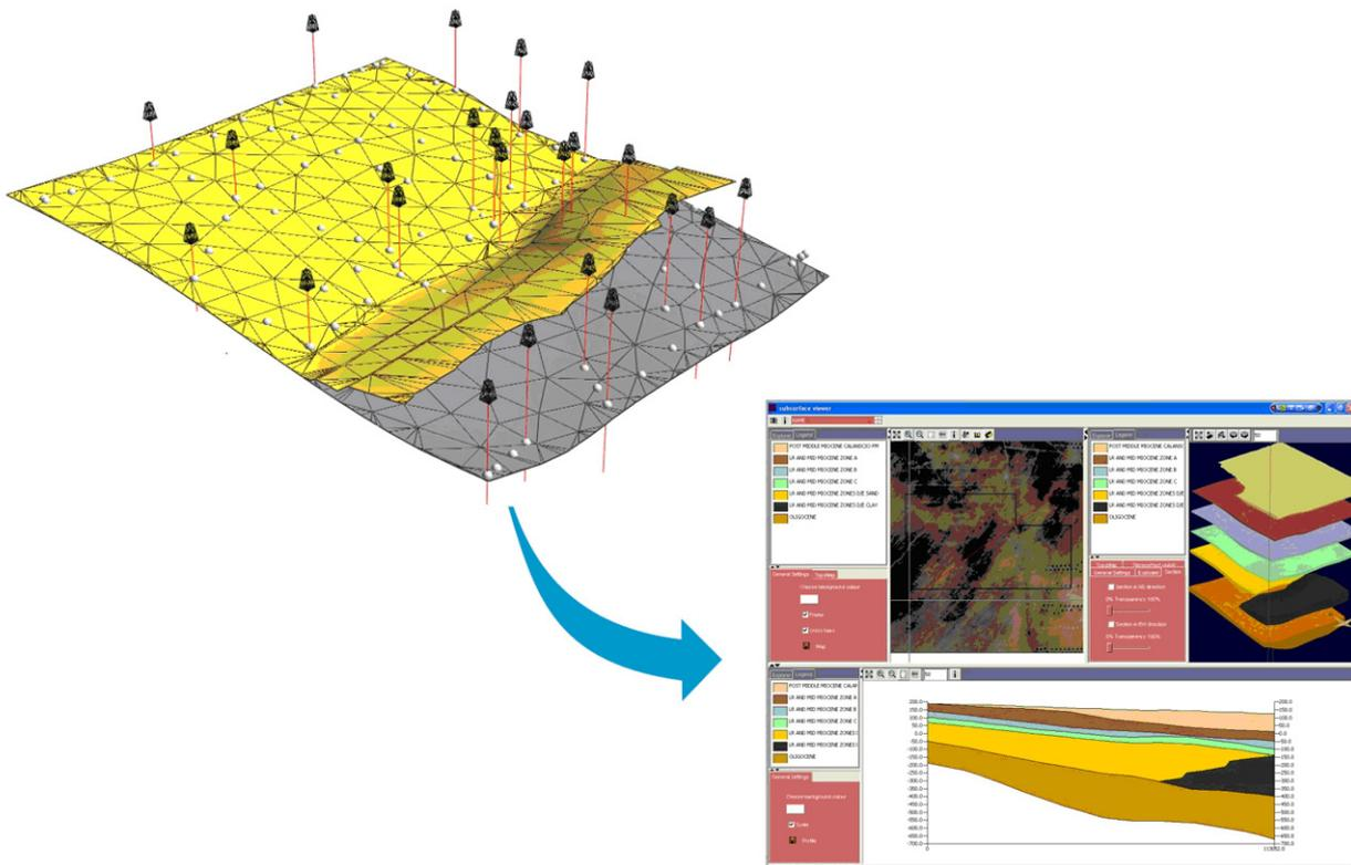
Figure 11 Triangulated surfaces in GOCAD exported to the Subsurface Viewer for delivery.
