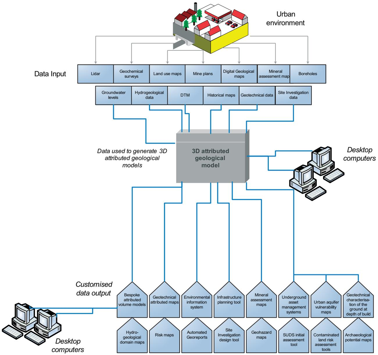
**Figure 6** Flow diagram showing the process of building and attributing the 3D geological model.
