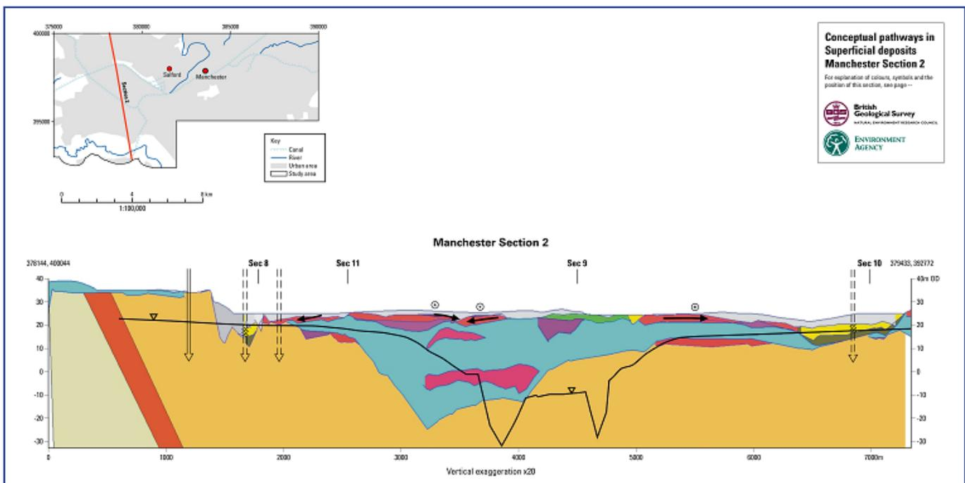
**Figure 5** GSI3D constructed section showing flow pathways and recharge from the EA Manchester urban study.
