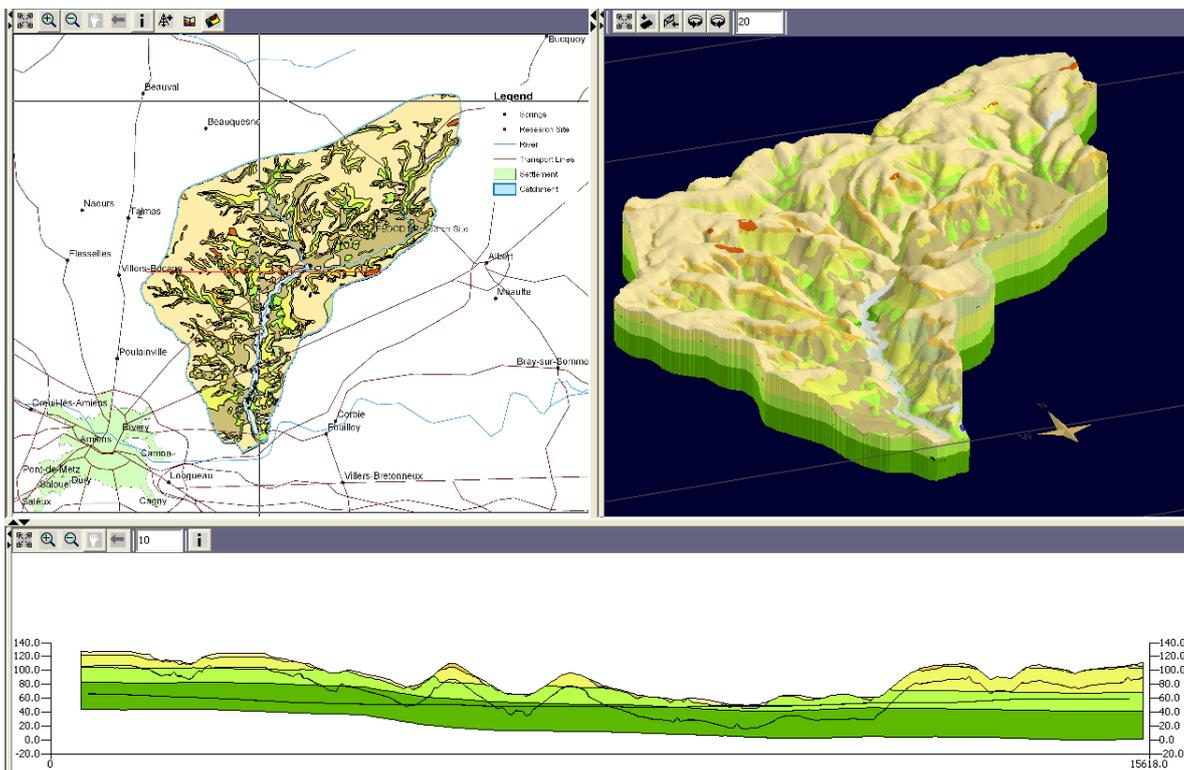
Figure 18 The Hallue 3D geological model in the subsurface viewer.
