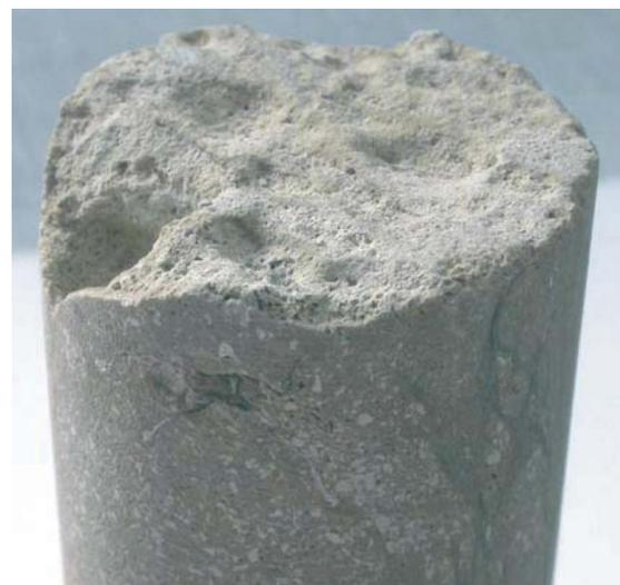
**Figure 17** The inlet end of sample GEUS 1 (Midale Marly Unit, M1 zone), before the CO<sub>2</sub> flooding experiment (top left), and after the experiment (top right and bottom right). Numerous small pits are present in the sample surface after the experiment. They represent dissolved calcite grains (peloids). The sample diameter is 2.48 cm.
