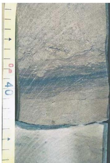
**Figure 4** An example of core material used in the flow and batch reaction experiments. A typical sample of the M1 Midale Marly Unit. This is an oil-stained dolostone with irregular, darker oil-stained shaly laminae. From Pearce and Springer (2001).
