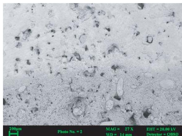
**Figure 21** Scanning electron photomicrograph of a monolith of the Midale Vuggy Unit, showing a well-developed 'tide mark' with increased dissolution within the water-rich phase (i.e. the lower half of the image). The sample had reacted for eight weeks with CO<sub>2</sub>.
