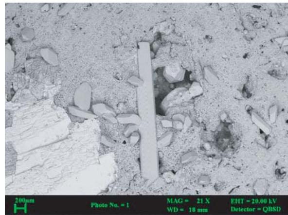
**Figure 22** Scanning electron photomicrographs of Midale Vuggy Unit monoliths showing well-developed secondary growth of gypsum crystals within the aqueous phase. After four weeks with  $\text{CO}_2$ , the crystals were up to  $500 \mu\text{m}$  long (left hand image), and after eight weeks they were at least  $2.5 \text{ mm}$  long (right hand image).
