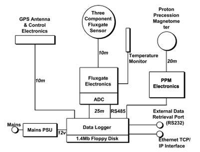
available for dissemination through either a network port, RS232 serial port or floppy disk. The processor and the sensors are powered by a single mains-voltage supply with a 24 hour battery reserve. The architecture of the operating system and the design of the acquisition software provide a versatility that allows new sensors to be readily incorporated such that
