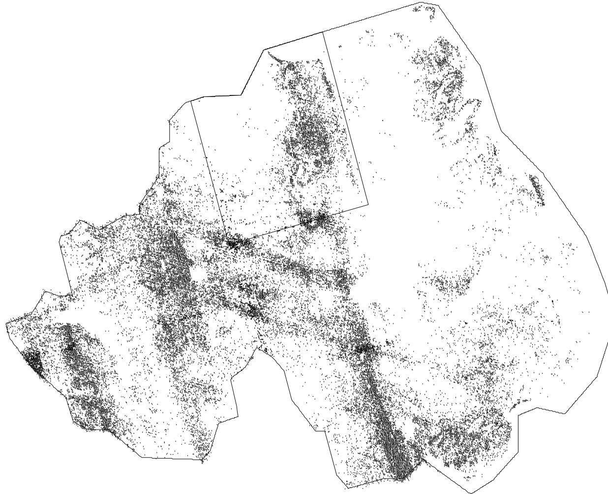
Figure 35. Plot of TELLUS survey flight lines over Northern Ireland showing line segments where ^{137}\text{Cs} > 2.7 \text{ kBqm}^{-2} . Block C from the 2005 survey outlined in black to demonstrate that band structure is not on the block boundary
