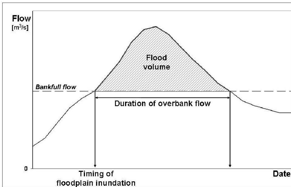
Figure 3.1 Parameters applied in this study to analyse floodplain inundation.
