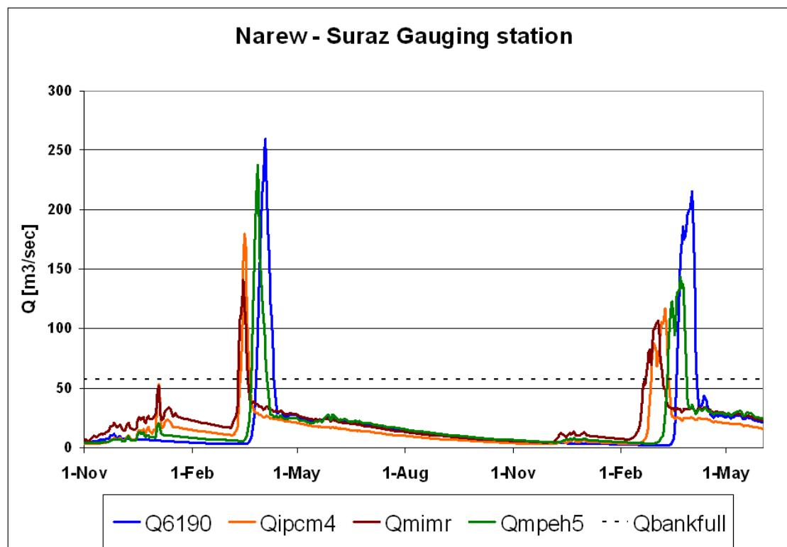
**Figure 3.6** Two year example of the Narew River in Poland simulated by WaterGAP showing changing discharges in the 2050s under the three applied scenarios compared to the baseline period (blue hydrograph).
