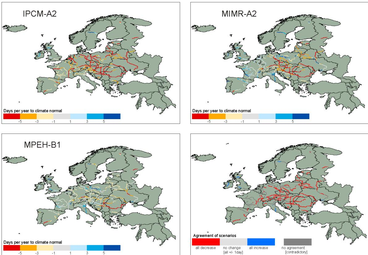
Figure 3.3 Change in duration of overbank flows in the 2050s compared to the baseline period (1961-90) under different future GCM-scenario combinations (IPCM4-A2, MIMR-A2 and MPEH5-B1). Agreement between these scenarios is shown in the map on the bottom right.
