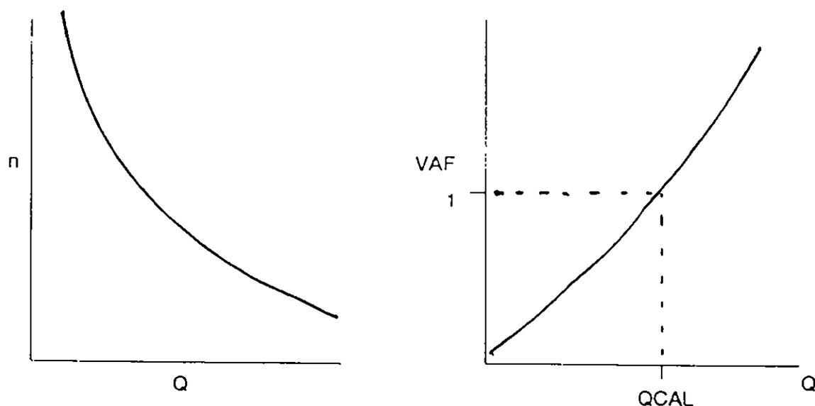
Figure 9: variation in *n* (roughness) and VAF with discharge
