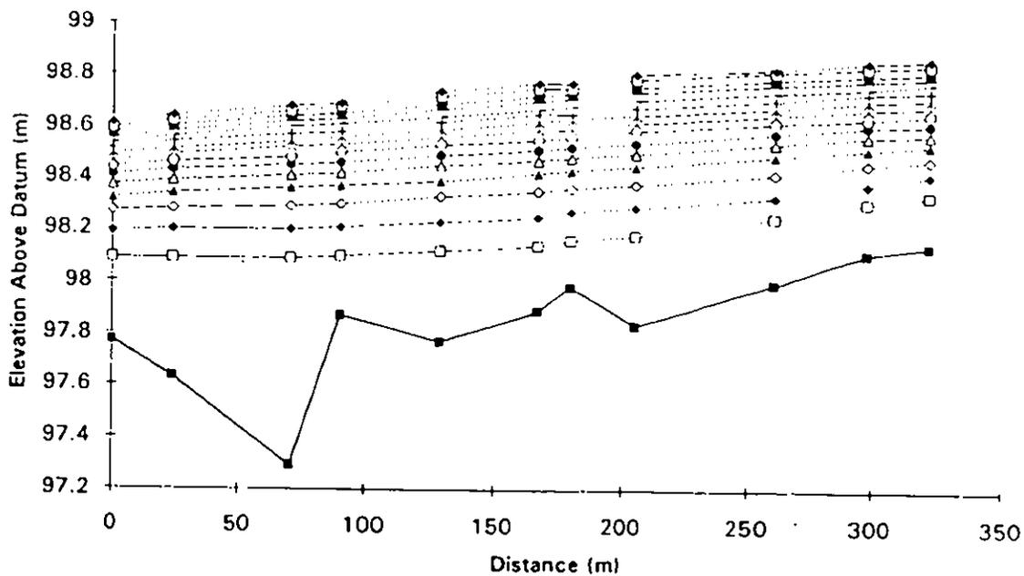
Figure 8: Complete range of simulated water surface levels
