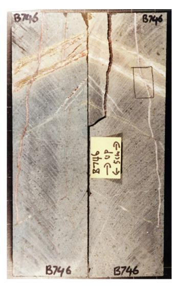
**Figure 14** Example description of filled discontinuities in a longitudinally sliced section of borehole core, 9 cm wide and 30 cm long in greyish green volcaniclastic rock. Acid etching and staining of the left-hand surface have been used to identify the carbonate minerals in fracture fillings.
