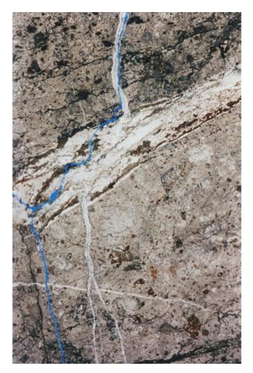
**Figure 18** Example description of filled discontinuities in a 2 x 3 cm area of blue-dye resin impregnated thin section prepared from altered volcaniclastic rock.
