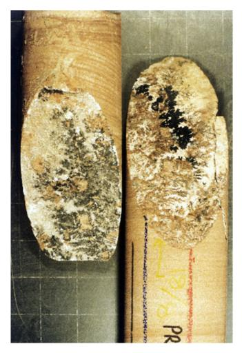
Figure 16 Example description of a filled discontinuity in borehole core.
