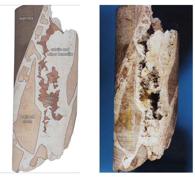
Figure 17 Example description of a partly filled discontinuity in borehole core.
