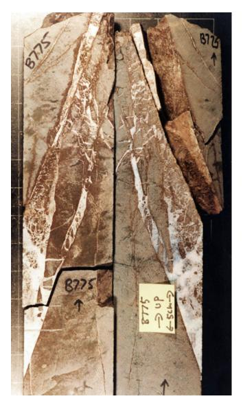
**Figure 15** Example description of filled discontinuities in a longitudinally sliced section of borehole core, 9 cm wide and 30 cm long, in greyish green volcaniclastic rock; acid etching and staining of the right-hand side has been used to help identify carbonate minerals in fractures.
