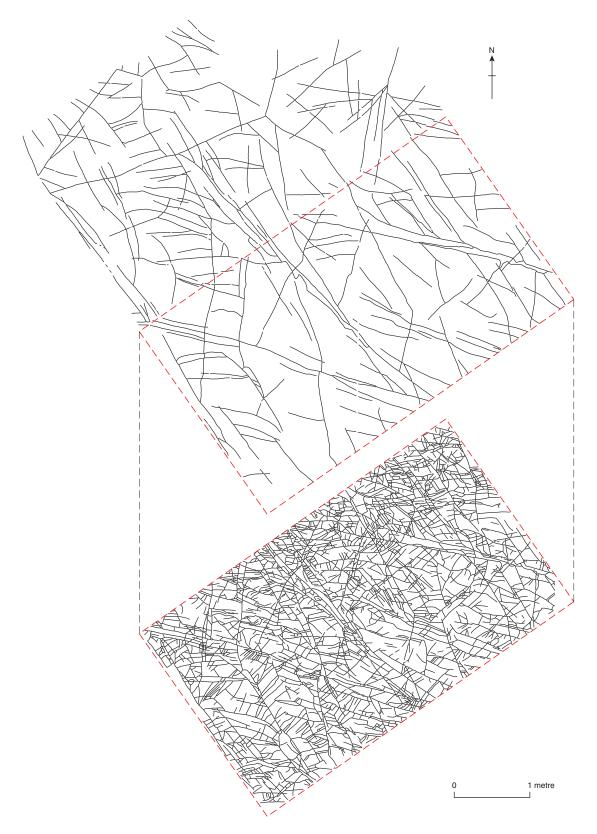
**Figure 8** Example trace map of a **discontinuity-network** displayed on a subhorizontal exposure surface in welded tuff, Gosforth, Cumbria. This example presents an illustration of the effect of a size cut-off for mapped features: in the upper diagram, only discontinuities greater than 50 cm long were mapped, while the lower diagram shows a trace map of all the discontinuities that can be discerned on the exposure surface within the area outlined by the dashed red line.
