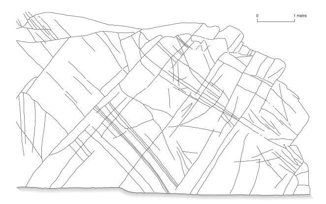
**Figure 9** Example trace map of a **discontinuity-network** displayed on a near-vertical exposure surface in a felsite intrusion, Gosforth, Cumbria. The face is inclined 84° south-south-east, and two discontinuity sets are evident: one has 10 cm- to m-range spacing, with an apparent dip to the west (left); in the other set, discontinuities with cm- to 10 cm-range spacing and a gentle/moderate apparent dip to the east form clusters with m-range spacing.
