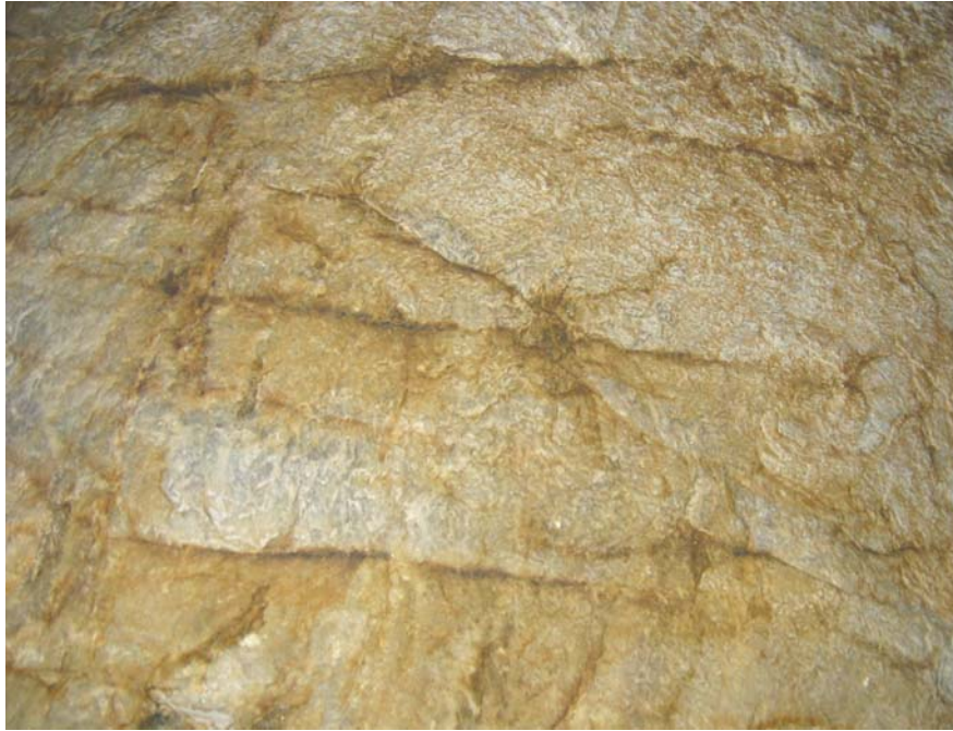
Figure 5 Stained but dry fractures are evidence of former groundwater movement
