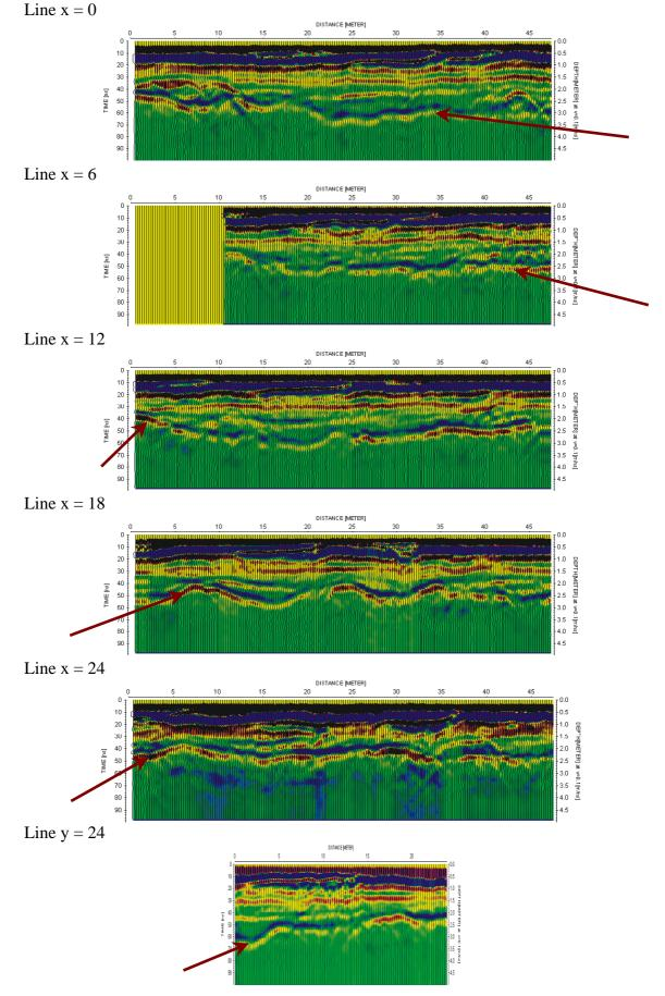
Figure 8. Radargrams of 100 MHz data from the '5 m bench' at Holme Pierrepont. Data were collected along five lines in the x direction and one line in the y direction. Depth conversion based on a velocity of 0.1 m ns<sup>-1</sup>. Mercia Mudstone reflector indicated by an arrow.
