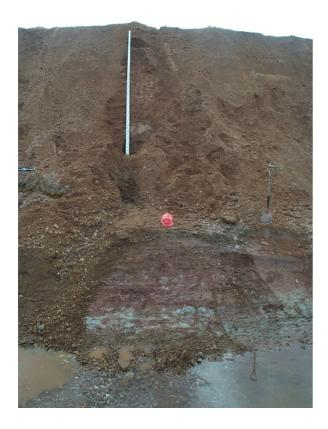
Figure 13. Approximately 4.9 m of gravelly sands (Holme Pierrepont Sand and Gravel) overlying very soft - firm red clays with very hard siltstone bands of the Gunthorpe Formation (Mercia Mudstone). Grey-green reduction zones can also be seen in the Mercia Mudstone. Vertical section at approximately x = 12, y = 0, on the '10m bench'.
