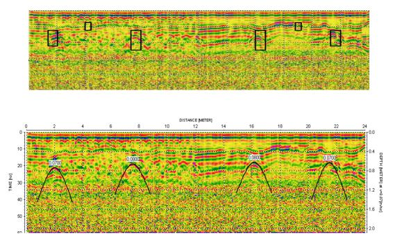
Figure 15. Radargram from the TRL road test track illustrating a number of features. The black squares in the upper image shows the location of voids. GPR hyperbolae from the voids are highlighted in the lower image where they have been used to estimate radar velocities.
