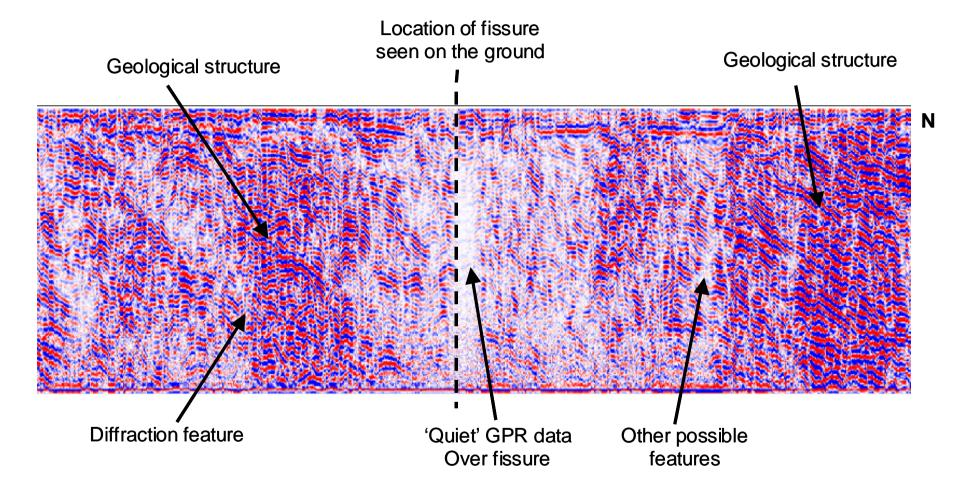
Figure 4. Summary of the general features seen at Houghton Hill farm. The fissure is shown as a shadow feature. Considerable geological structure is observed. Other shadow zones may suggest smaller scale fissures. A diffraction feature is also seen at depth and could also be a fissure. Assuming a radar velocity of  $0.0715 \text{ m ns}^{-1}$ , the section has a full depth extent of 7m.
