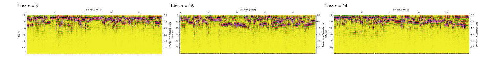
Figure 10. Radargrams of 250 MHz data from the '10 m bench' at Holme Pierrepont. Data are shown for every other line in the x direction. Depth conversion based on a velocity of  $0.1 \text{ m ns}^{-1}$ .
