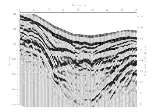
Figure 1. Example of a wiggle trace radargram. The reflections are interpreted as a kettle hole infilled with flat-lying onlapping sediments (after Busby and Merritt, 1999).
