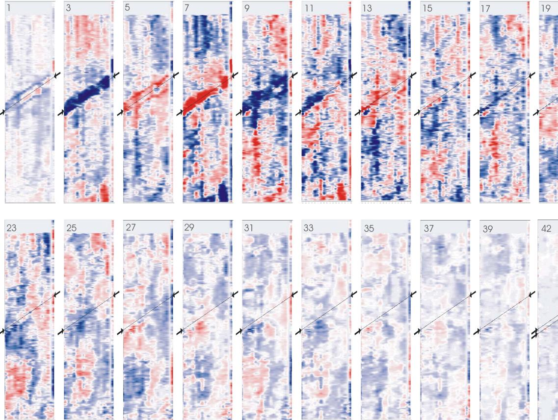
Figure 3. Time slices of GPR generated from a 3D data representation. Each successive map represents increasing depth. The location of the known fissure is highlighted. Depth slices from 1 to 42 represent the surface level down to a depth of approximately 1m, assuming a radar velocity of 0.0679 m ns<sup>-1</sup>.
