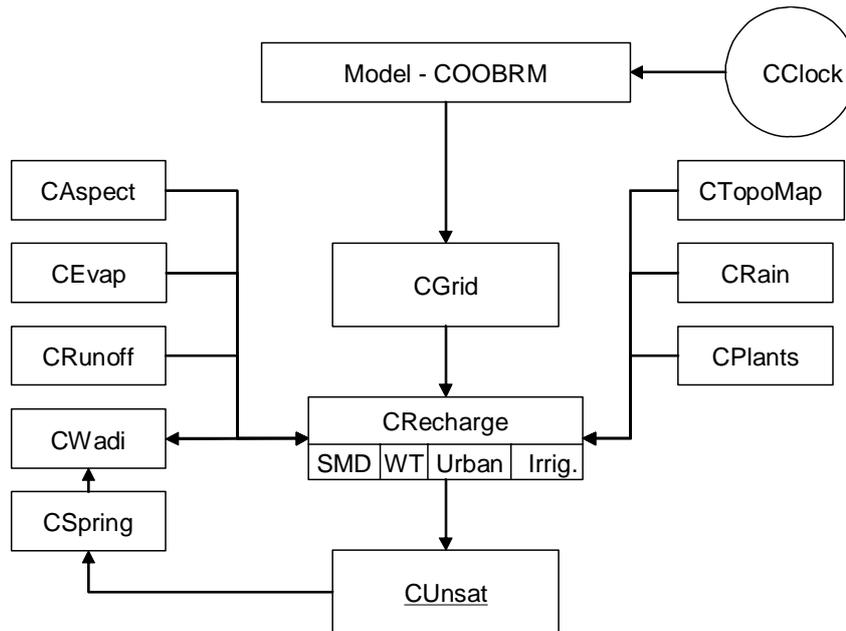
Figure 7 Framework of recharge model
