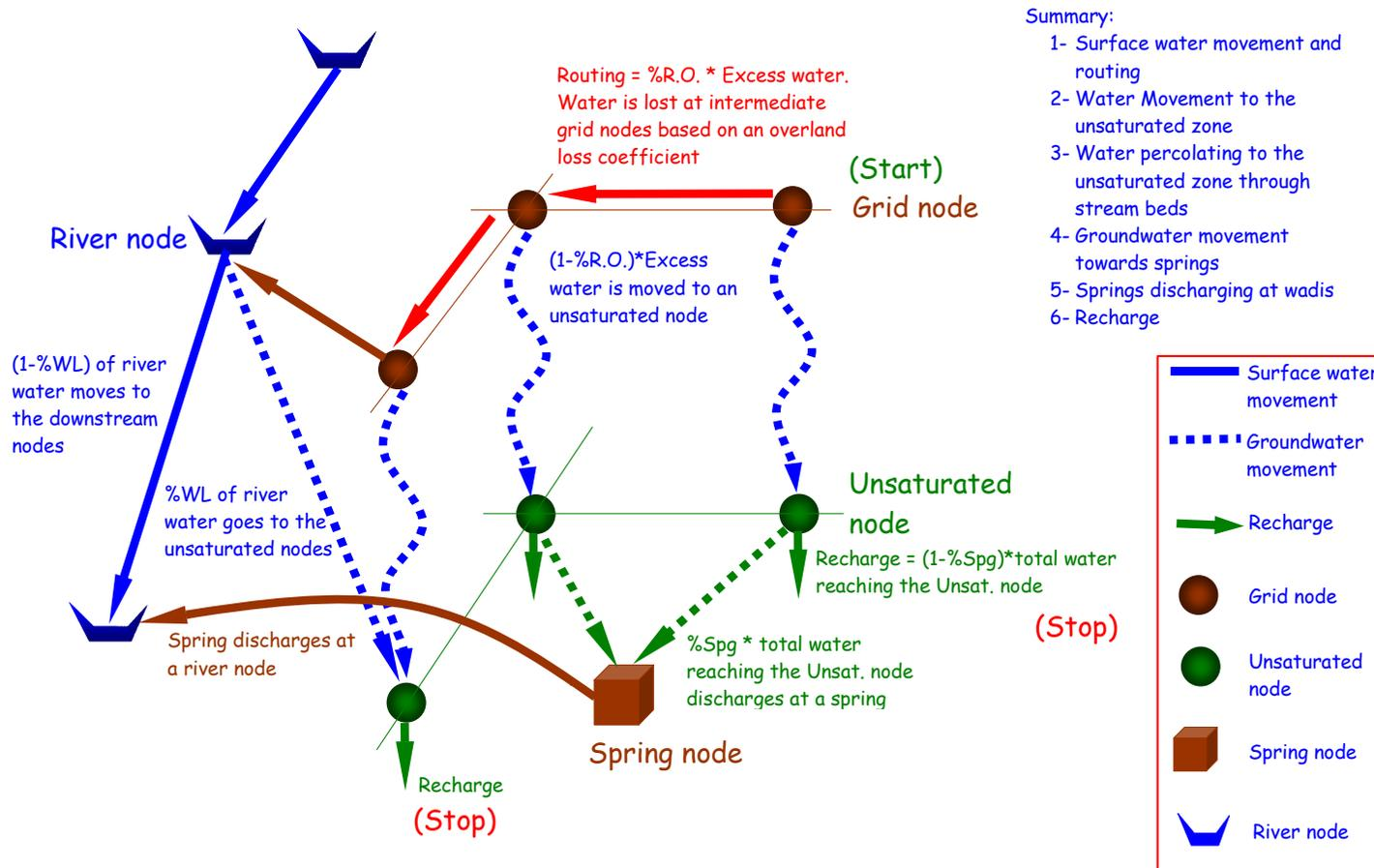
Figure 8 Outline of the calculation procedure
