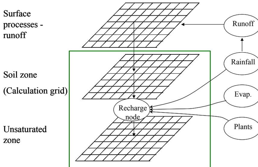
Figure 5 Relationship between grids in the recharge model
