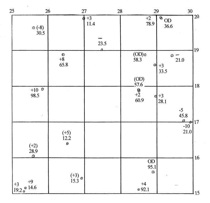
Figure 4 : Water wells proving Upper Chalk. The lower figure indicates the thickness of Upper Chalk penetrated. The upper figure indicates the OD level of the top of the Upper Chalk; where it is in brackets, the Upper Chalk is *not* overlain by Crag.
