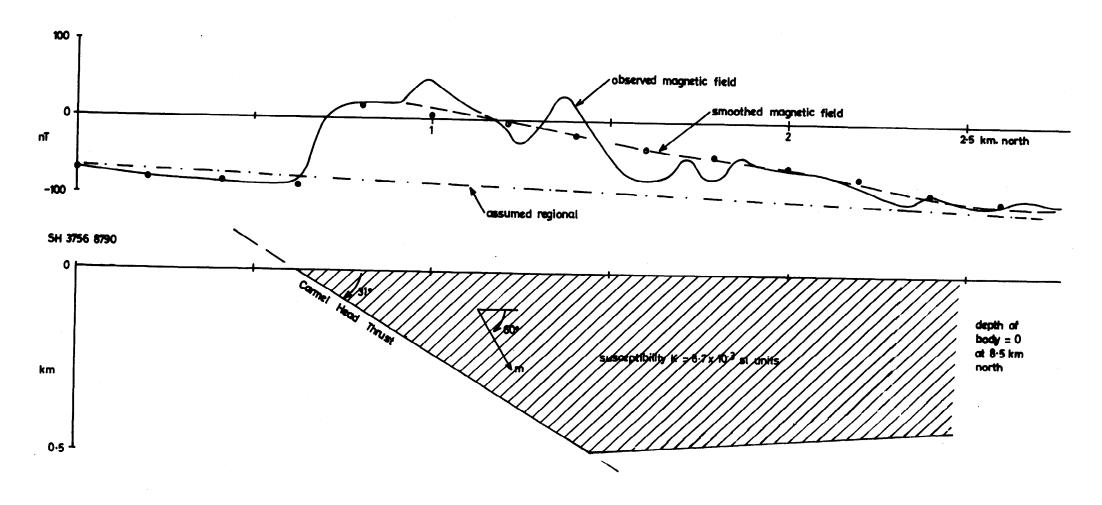
FIG. 4 SOUTH-NORTH TOTAL FIELD MAGNETIC INTENSITY PROFILE OVER CARMEL HEAD THRUST WITH INTERPRETED MODEL
